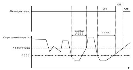
When setting F S G I = I (Tripping), inverter trips (U E G G) after low-current / torque is detected for the period of time set with F S G G G. Then, alarm signal remains ON.
