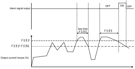
When setting  $F \subseteq G : I = I$  (Tripping), inverter trips  $(G \not E \not G : I)$  after over-current / torque is detected for the period of time set with  $F \subseteq G \subseteq I$ . Then, alarm signal remains ON.
