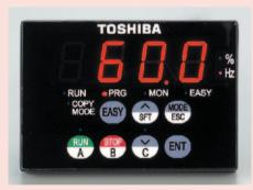
Our customers require a "display that is easily visible from a long way away." In response to this need, we developed this panel using 20 mm LEDs, the largest in its class in the market, to ensure outstanding visibility.
