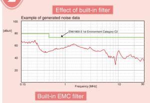
• High-frequency noise is drastically reduced on models with built-in noise filters. Built-in noise filters are ideal for sites from commercial facilities and offices through to factories where attention must be paid to peripheral devices.
