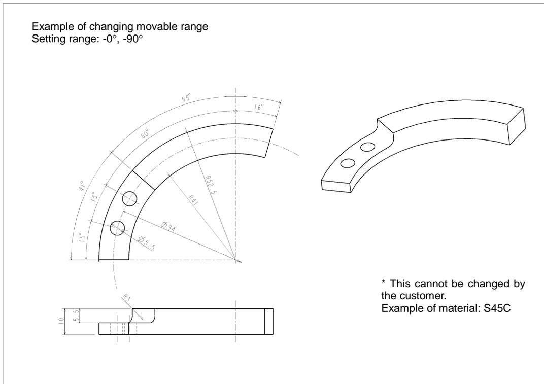
Fig. 3.24 Design example of mechanical stopper on the arm 2 (1) side (For reference, e.x. TVL500)
