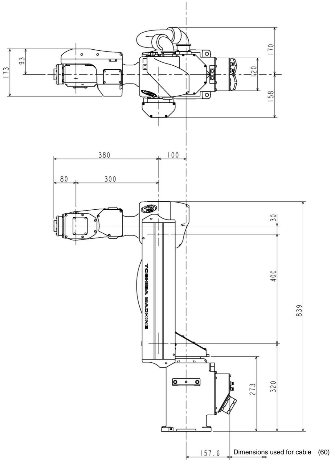
Fig. 1.6 External dimensions of the TVL700
