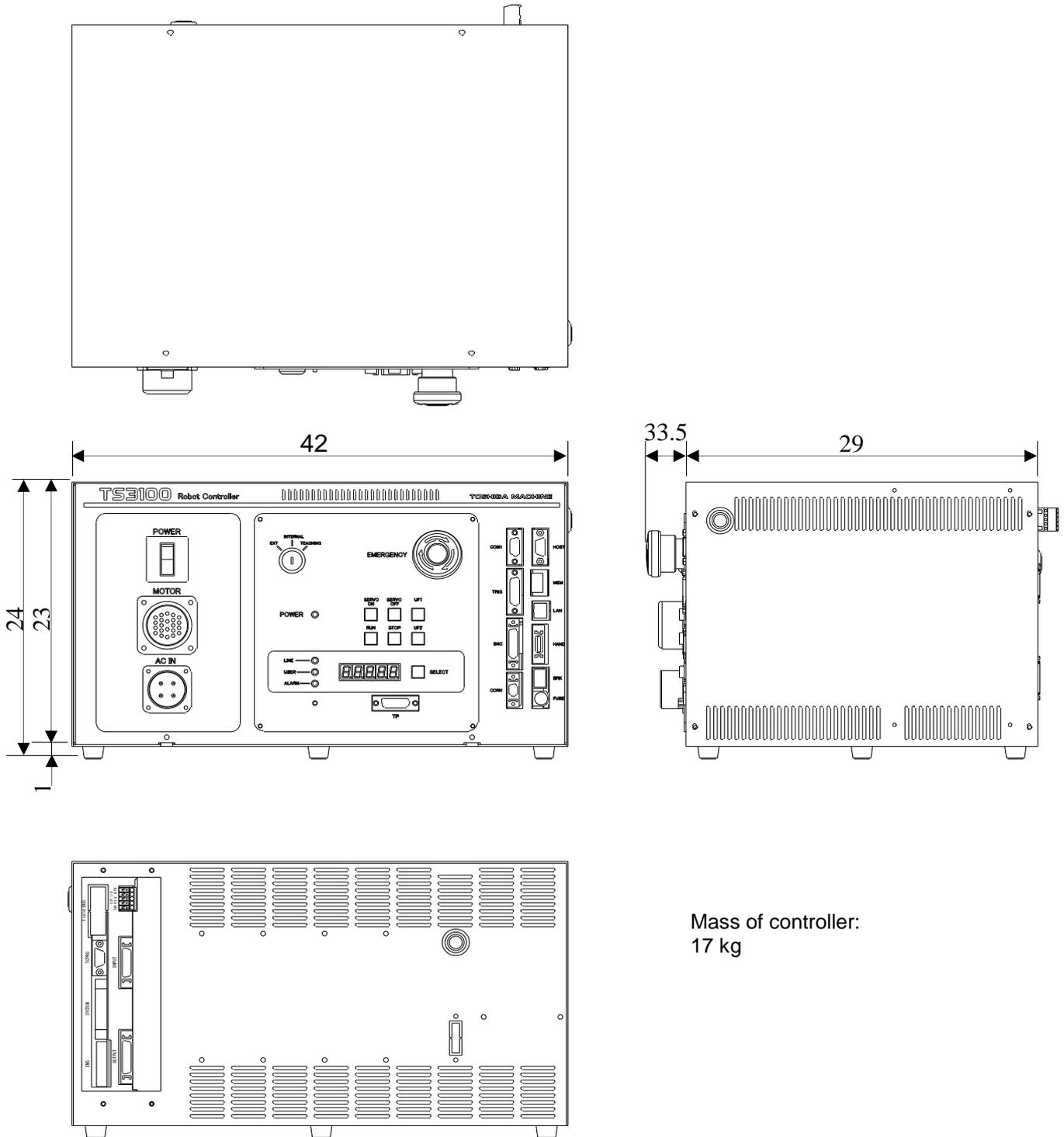
Fig. 6.1 External view of the controller(TS3100)
