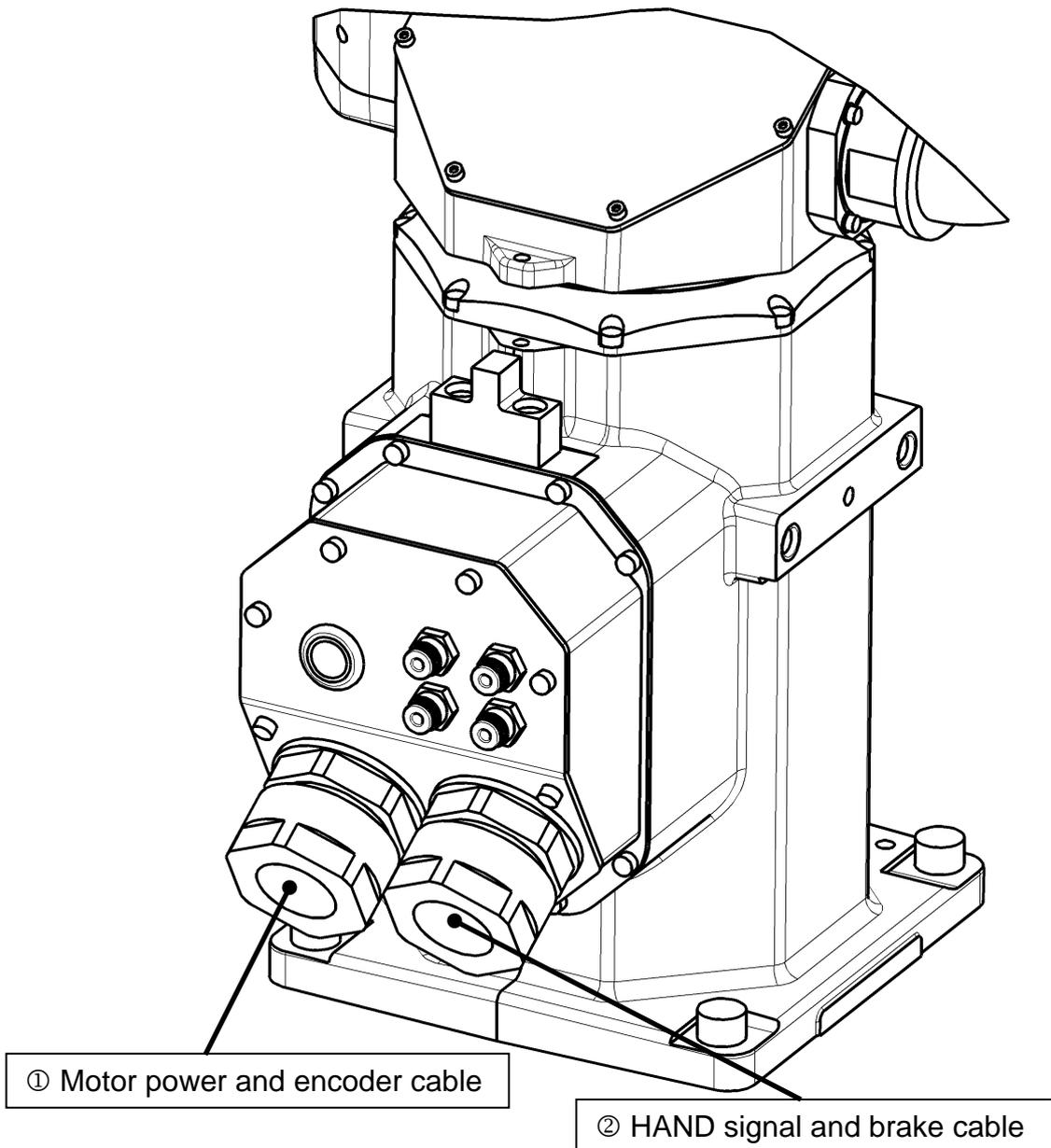
Fig. 8.2 Robot side connector arrangement (TSL3100E)
