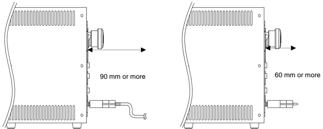
Fig. 6.5 Clearance in front of the Controller
