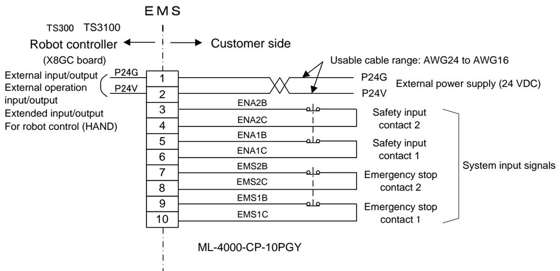
Fig. 9.3 Connection of External Power Supply (TS3100)
