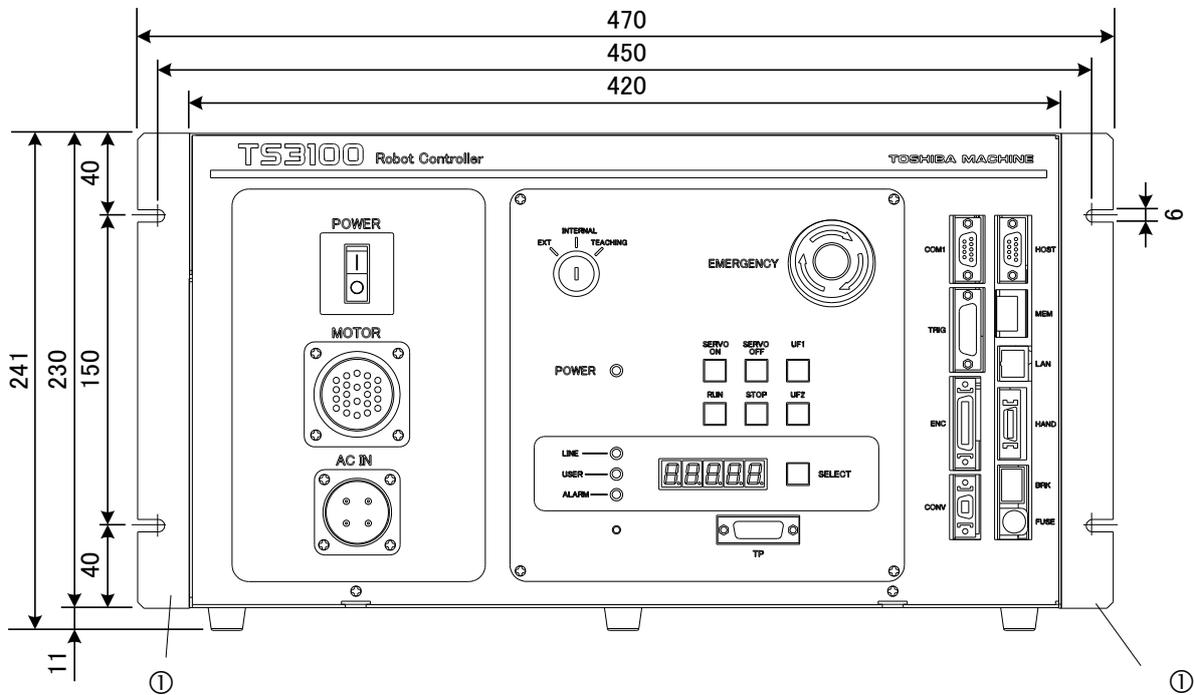
Fig. 6.3 Screw hole dimensions for securing controller
