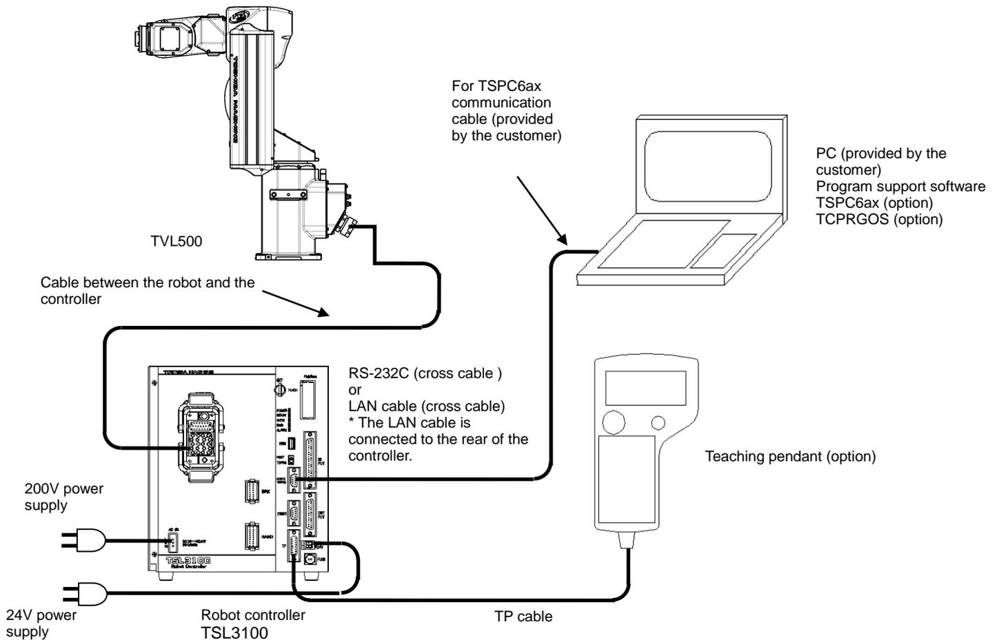
Fig. 1.1 Equipment Configuration (TSL3100)
