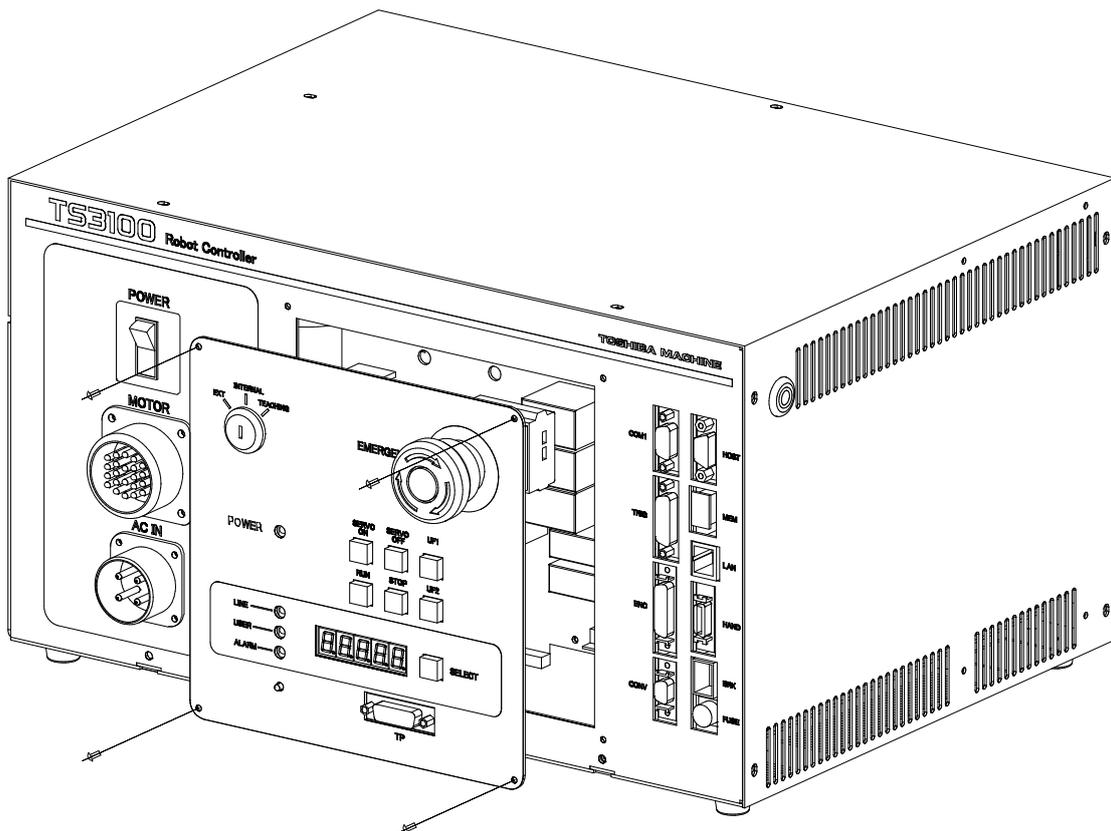
Fig. 9.6 Dismounting the control panel (TS3100)
