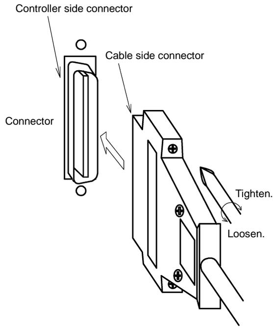
Fig. 7.4 Connecting and disconnecting a square connector (TSL3100)
