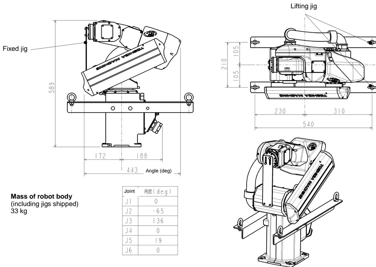
Fig. 2.3 Outer dimensions at transport
