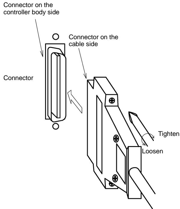
Fig. 9.5 Connecting and disconnecting a square connector (TS3100)
