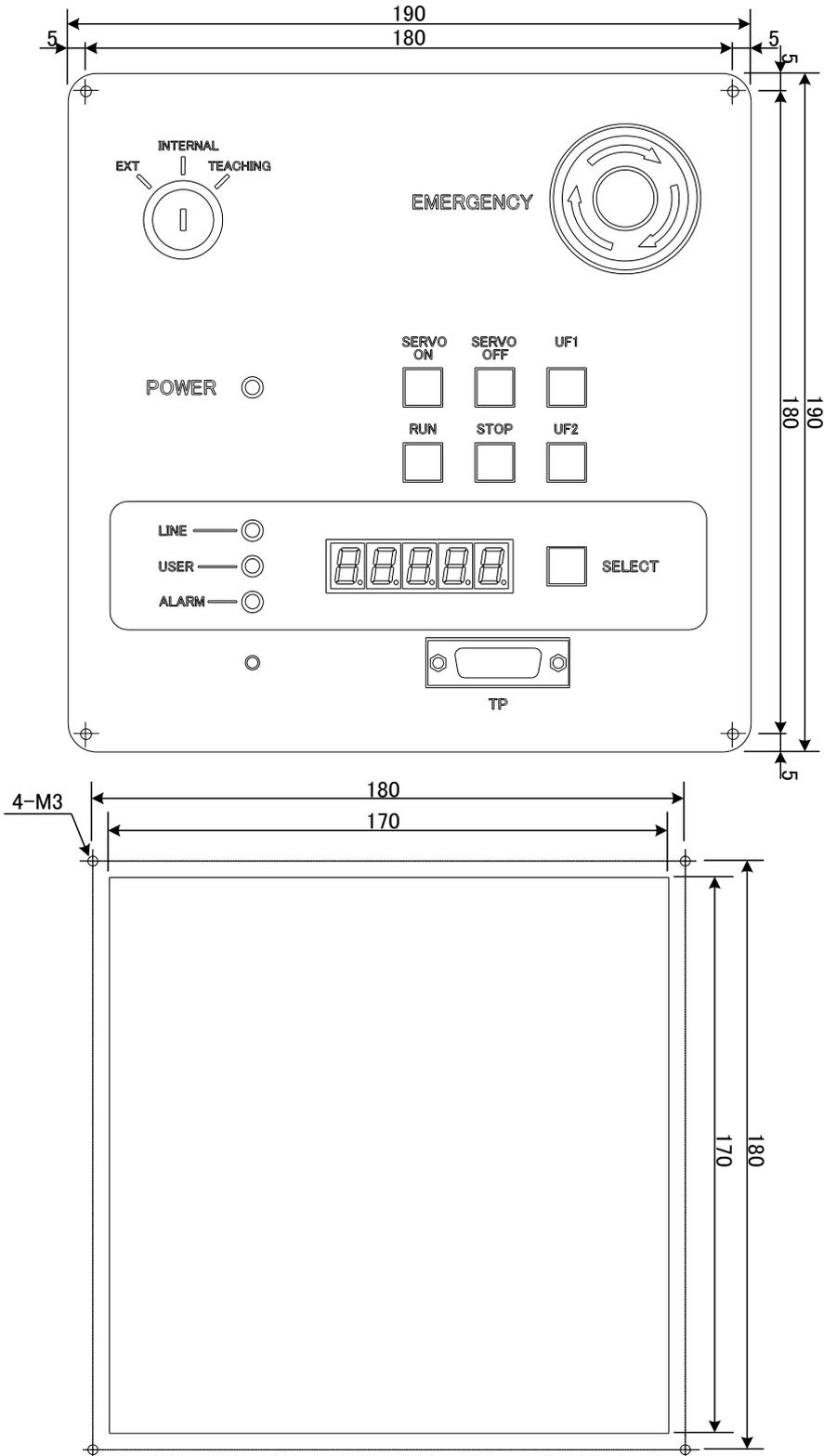
Fig. 9.7 Installation dimensions of the control panel (TS3100)
