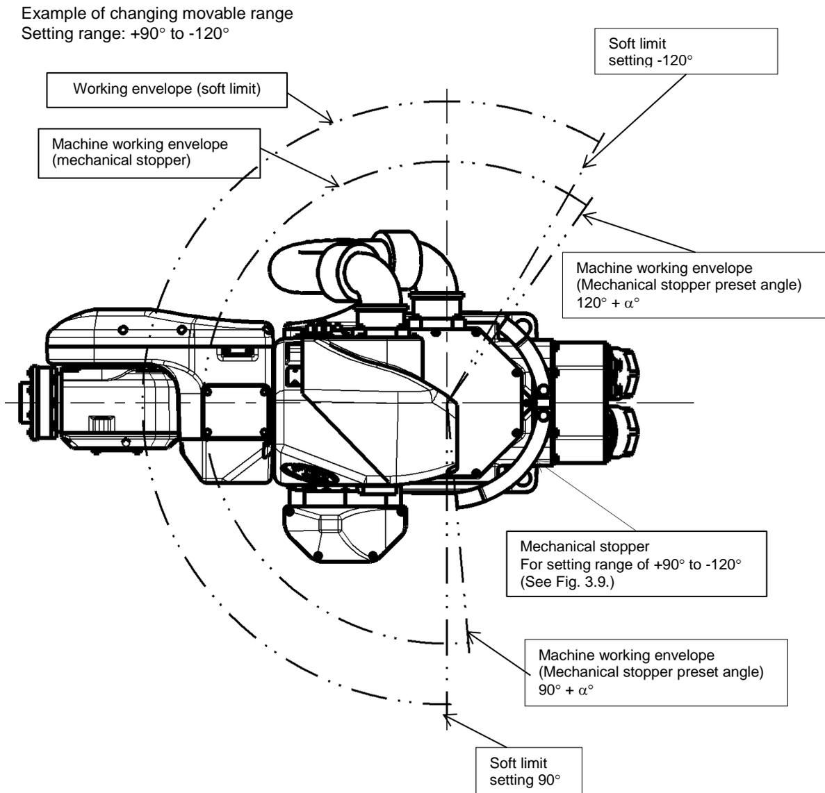
Fig. 3.11 Example of changing axis-1 working envelope (TVL500)
