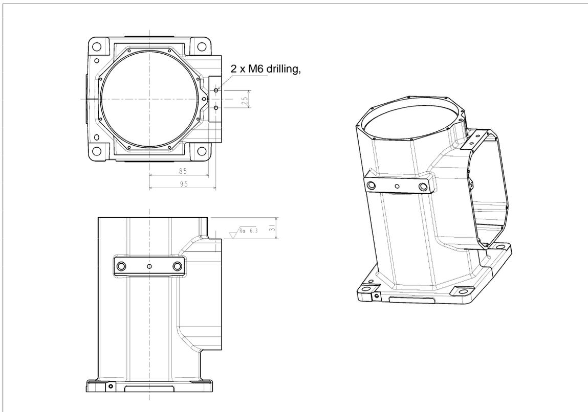
Fig. 3.10 Mechanical stopper location (at the base) (TVL500/TVL700)
