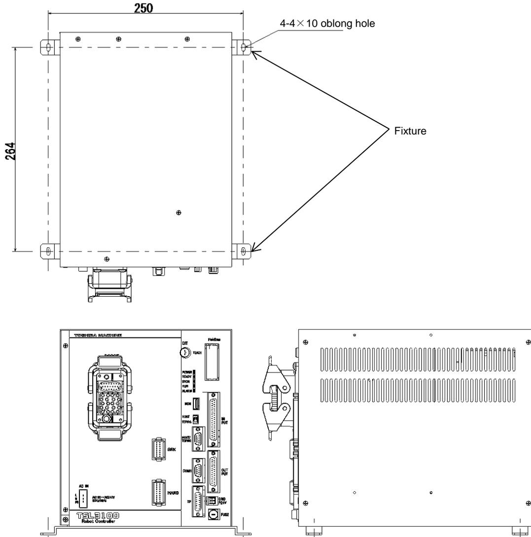
Fig. 4.3 Screw hole dimensions for securing controller (TSL3100)
