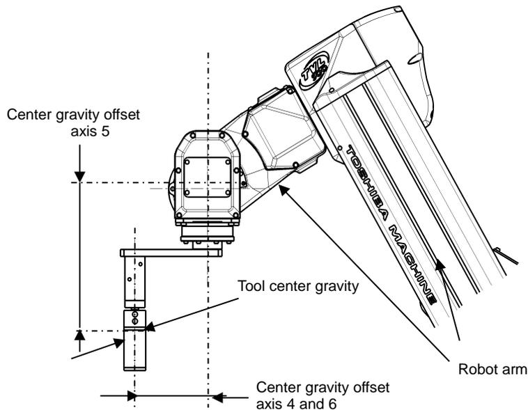
Fig. 10.4 Explanation of inertia moment
