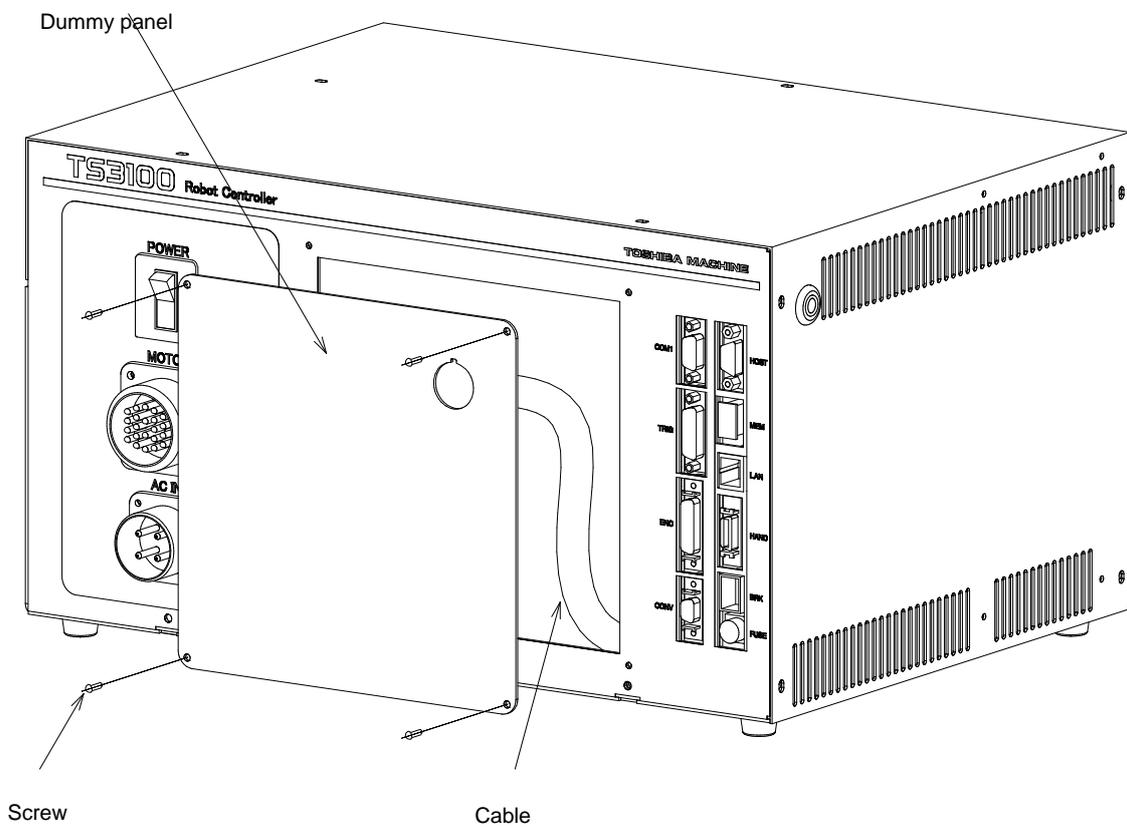
Fig. 9.8 Mounting the dummy panel (TS3100)
