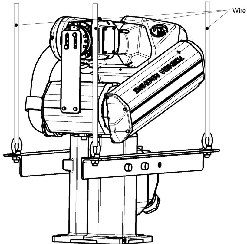
Fig. 2.5 Lifting up the robot (TVL500)
