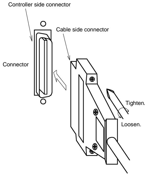
Fig. 8.4 Connecting and disconnecting a square connector (TSL3100E)
