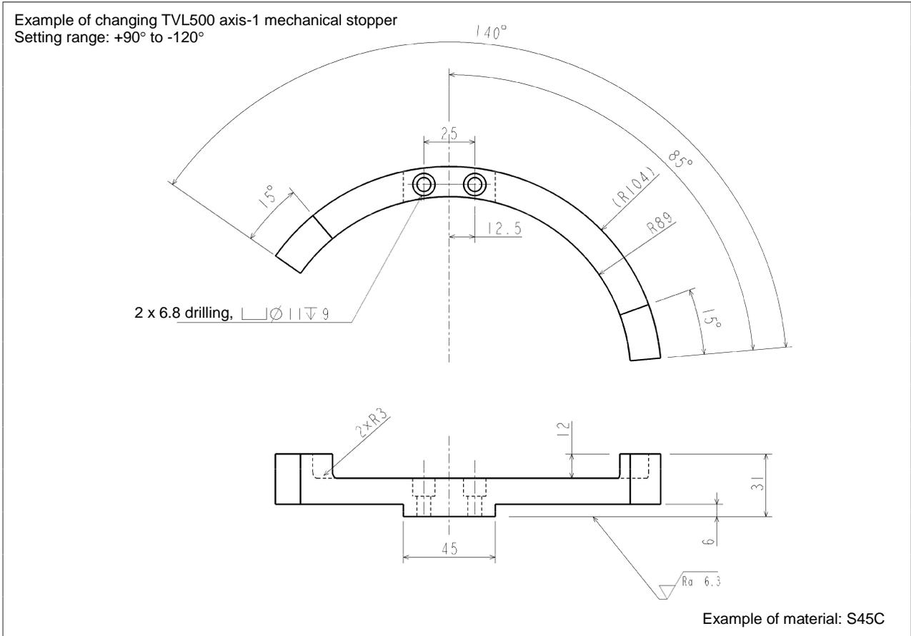
Fig. 3.12 Example of changing axis-1 mechanical stoppers (reference)
