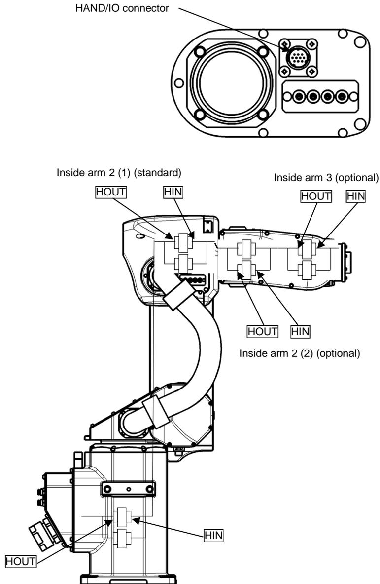
Fig. 12.2 Tool I/O wiring
