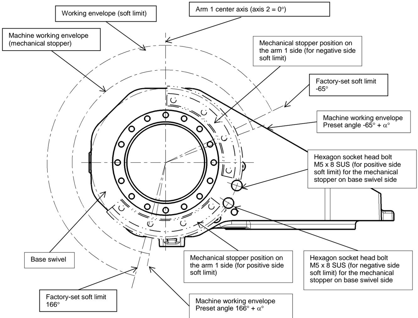
Fig. 3.13 Axis-2 working envelope setting (TVL500)
