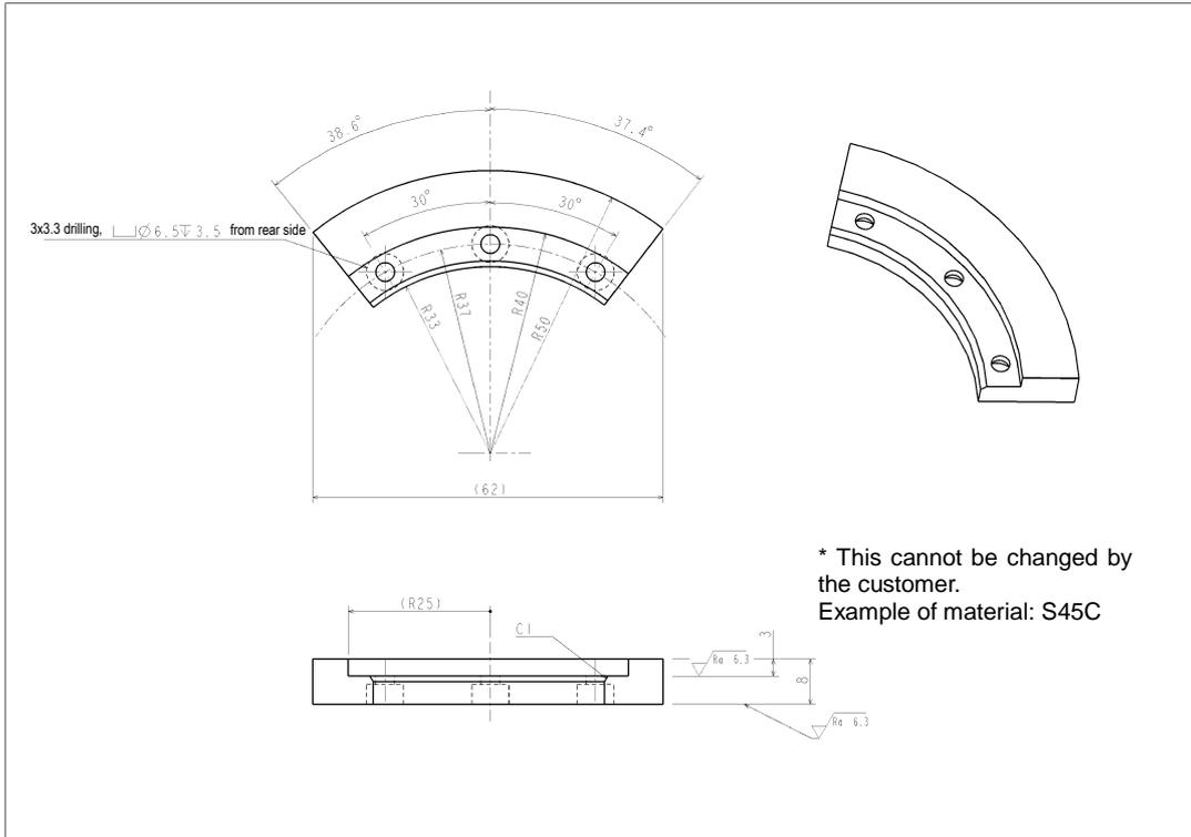
Fig. 3.22 Arm 1 side mechanical stopper (TVL500)
