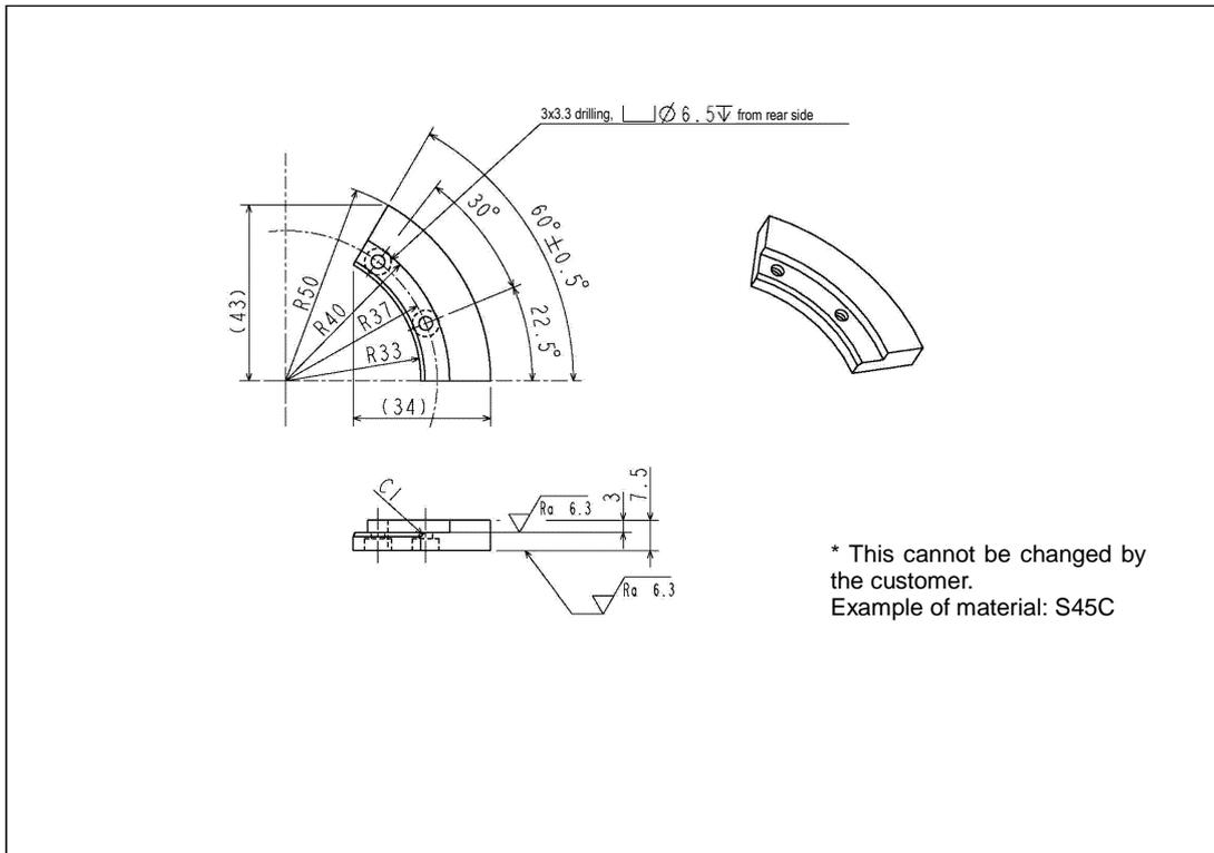
Fig. 3.23 Arm 1 side mechanical stopper (TVL700)
