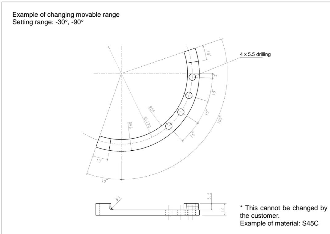
Fig. 3.18 Design example of mechanical stopper on base swivel side
