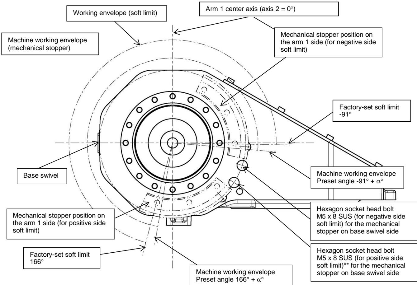
Fig. 3.14 Axis-2 working envelope setting (TVL700)
