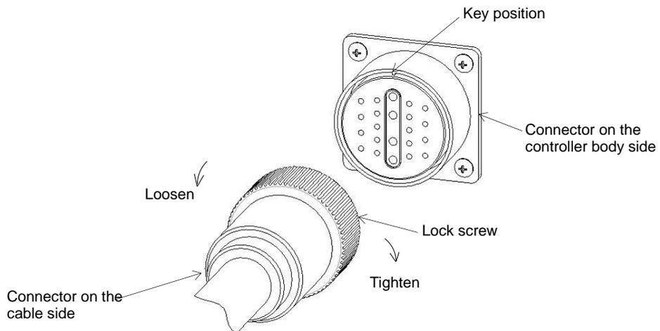
Fig. 8.4 Connecting/disconnecting the circular connector (TS3100E)
