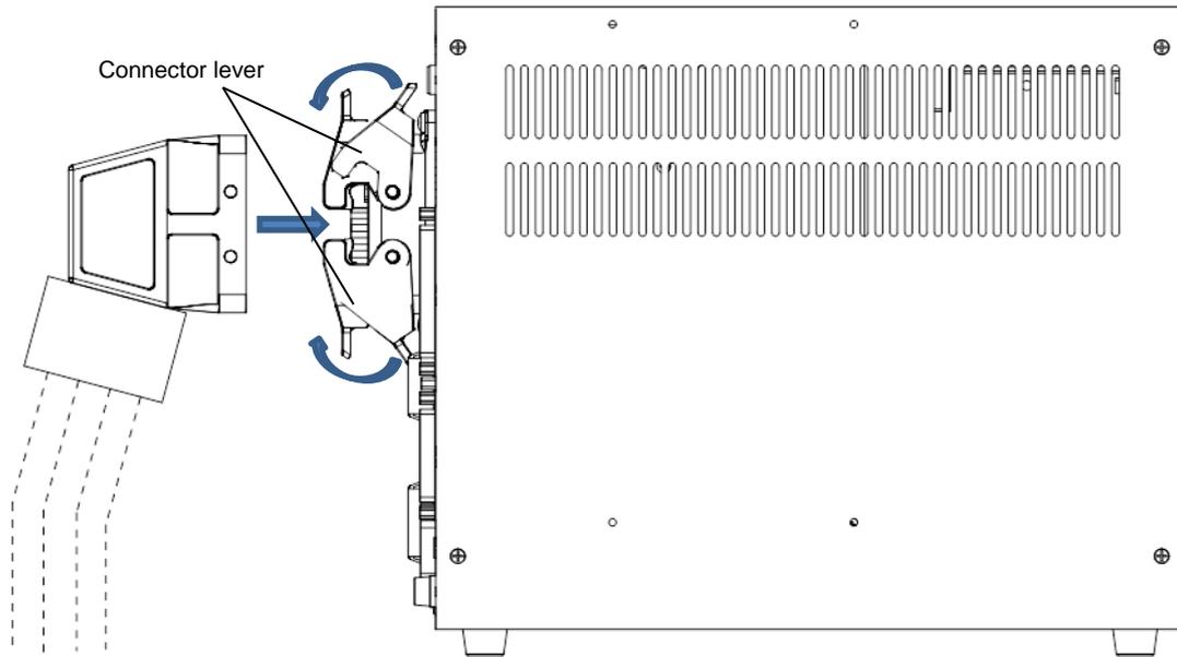
Fig. 8.3 Connecting and disconnecting a ROBOT connector(TSL3100E)
