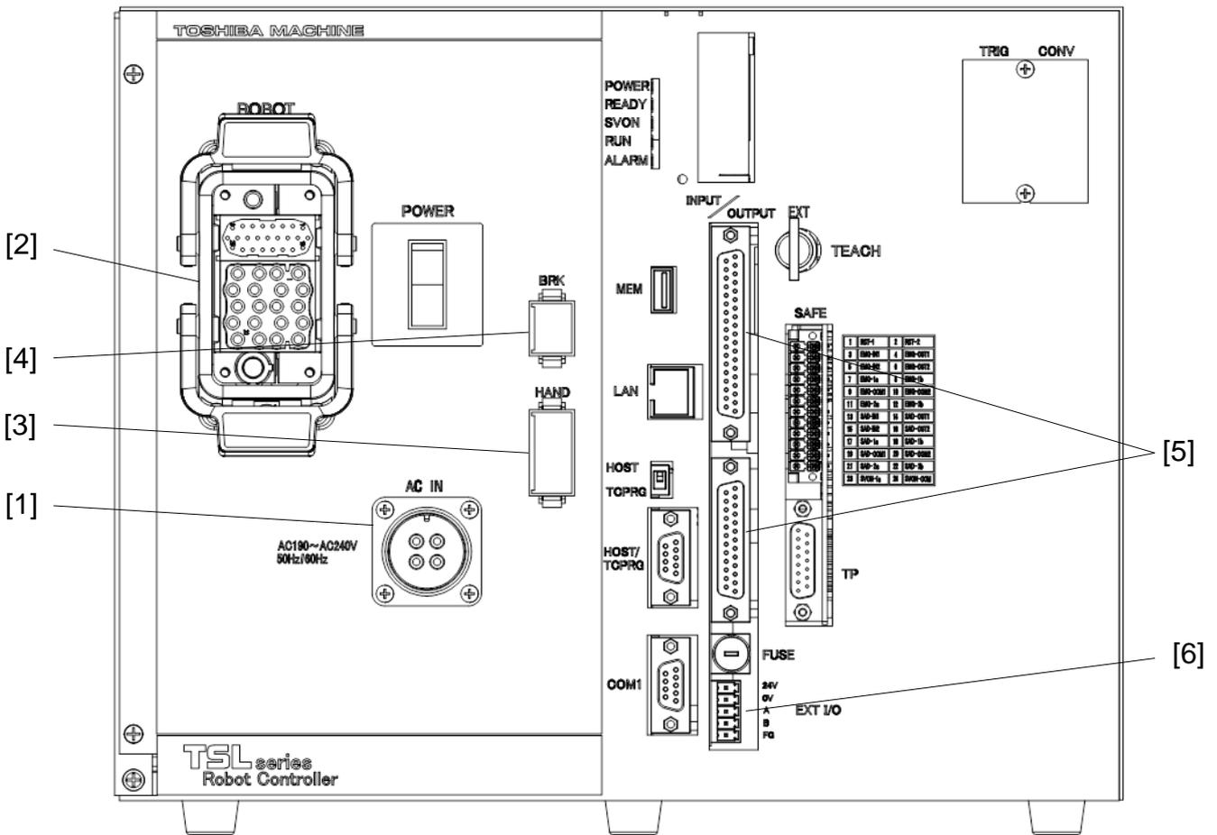
Fig. 8.1 Robot controller connector arrangement (TSL3100E)
