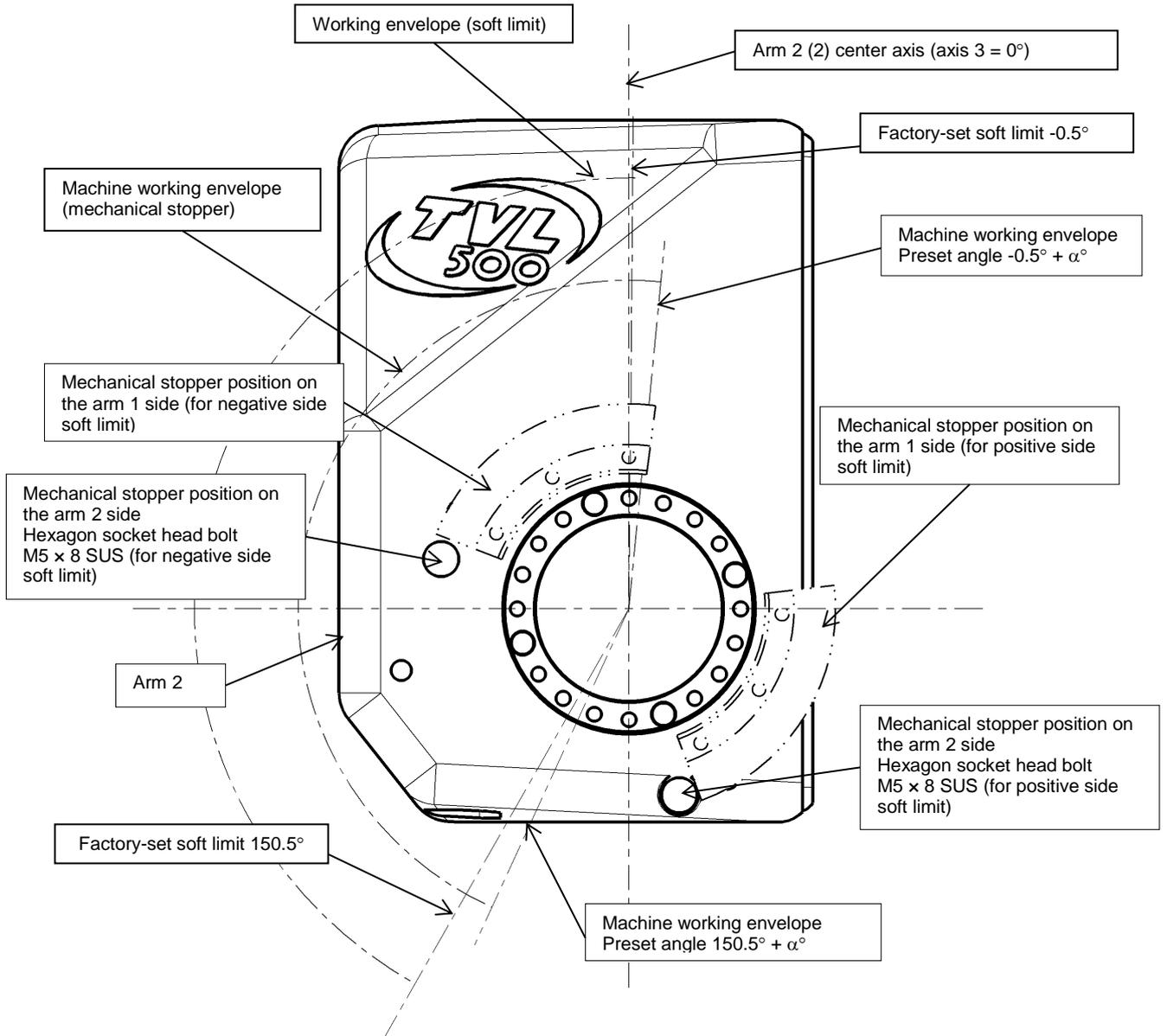
Fig. 3.19 Axis-3 working envelope setting (TVL500)
