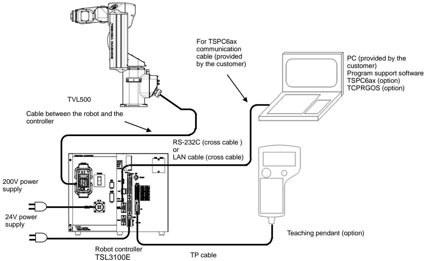
Fig. 1.2 Equipment Configuration (TSL3100E)
