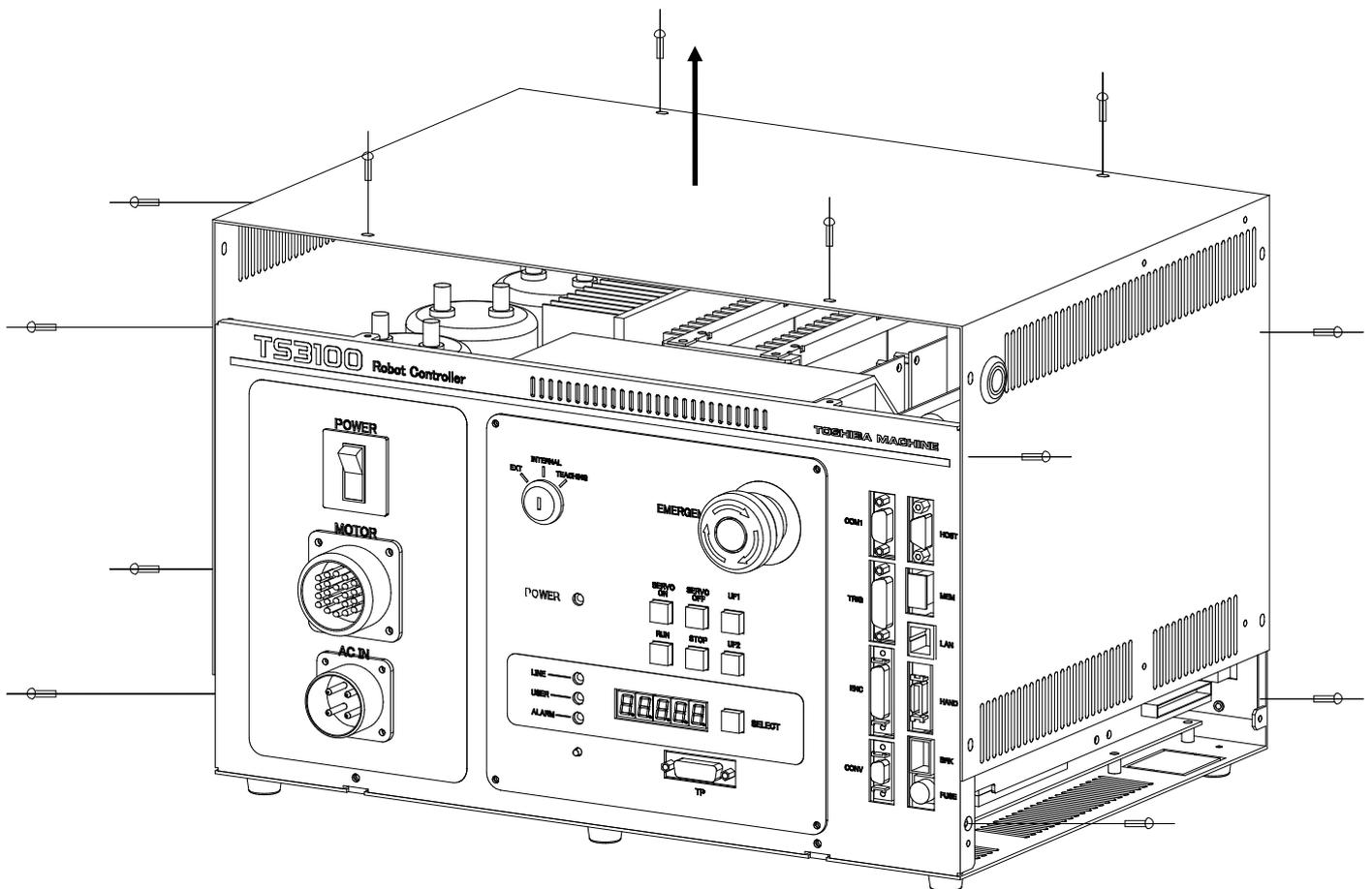
Fig. 6.4 Removing the upper cover
