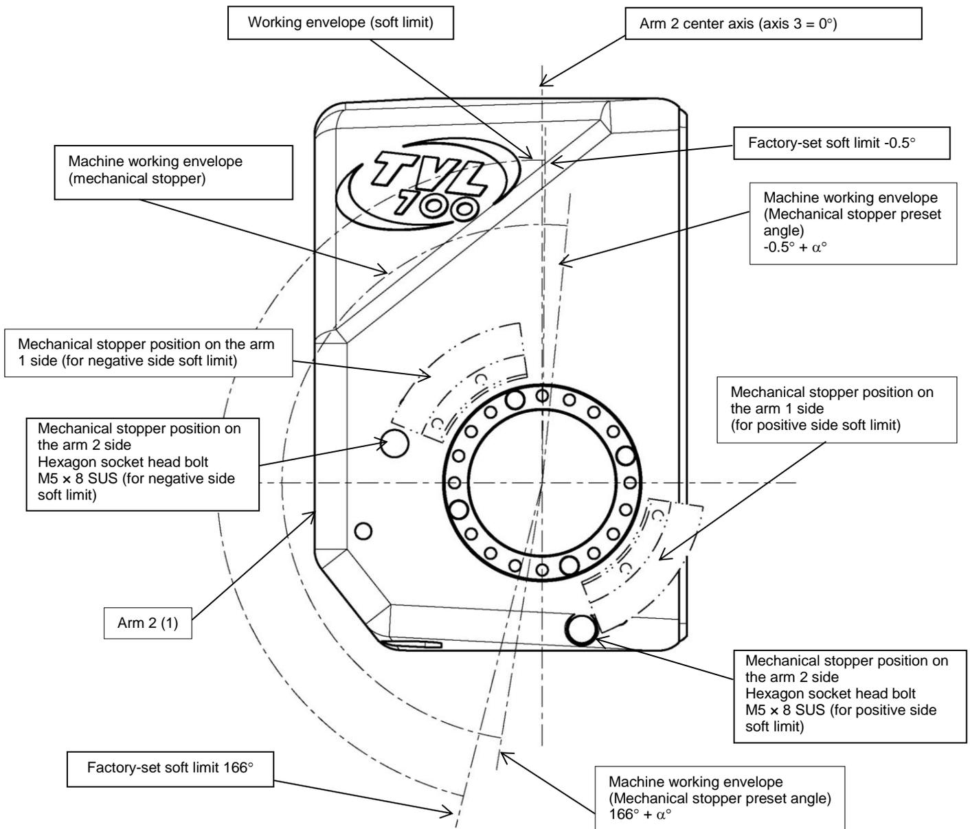
Fig. 3.20 Example of changing axis-3 working envelope (TVL 700)
