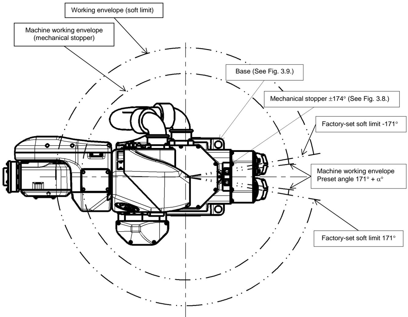
Fig. 3.8 Axis-1 working envelope setting
