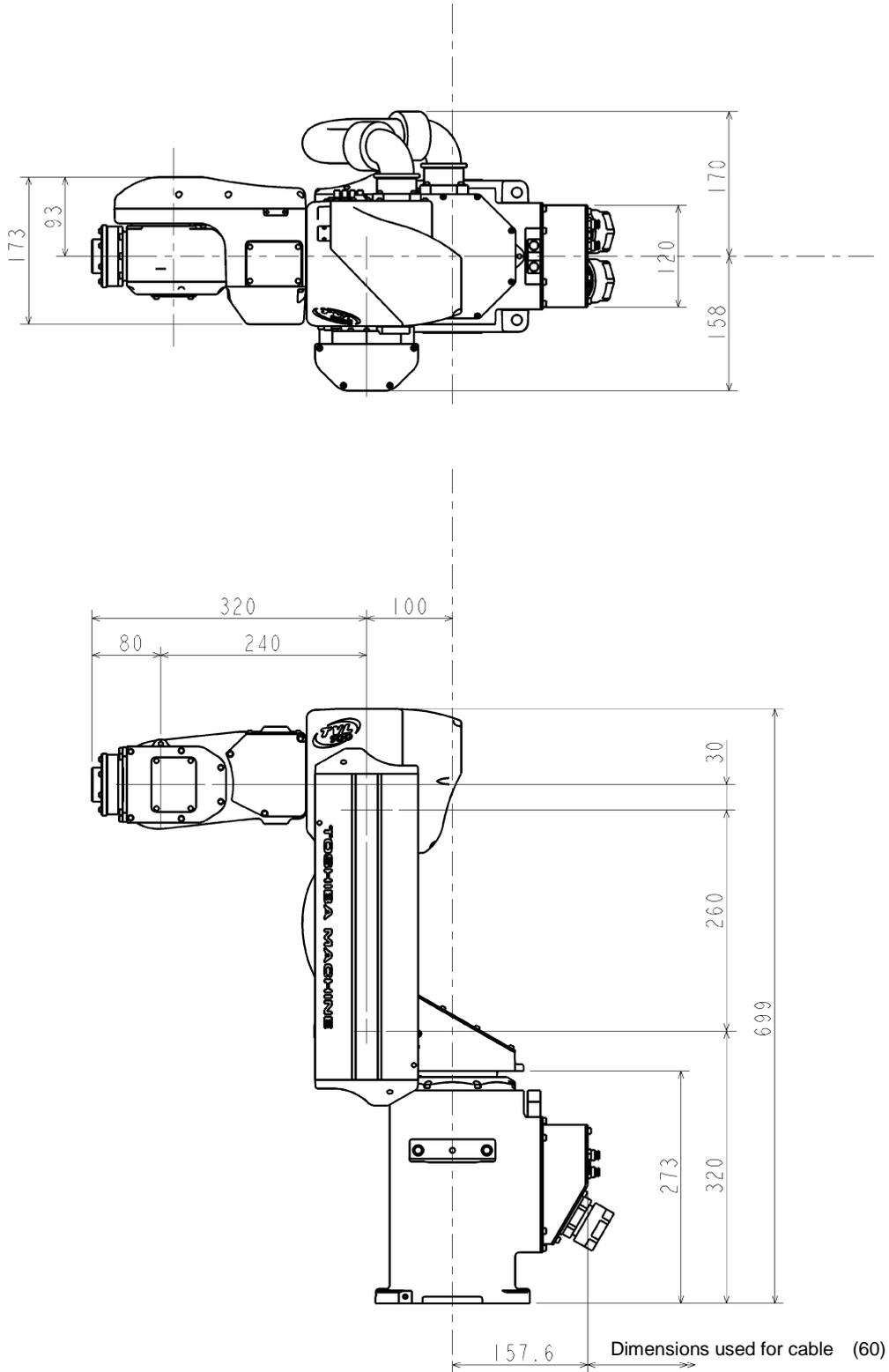
Fig. 1.5 External dimensions of the TVL500
