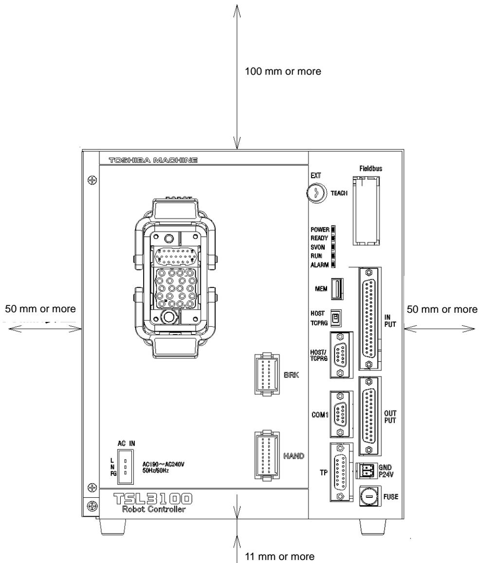
Fig. 4.2 Controller ventilation space (TSL3100)
