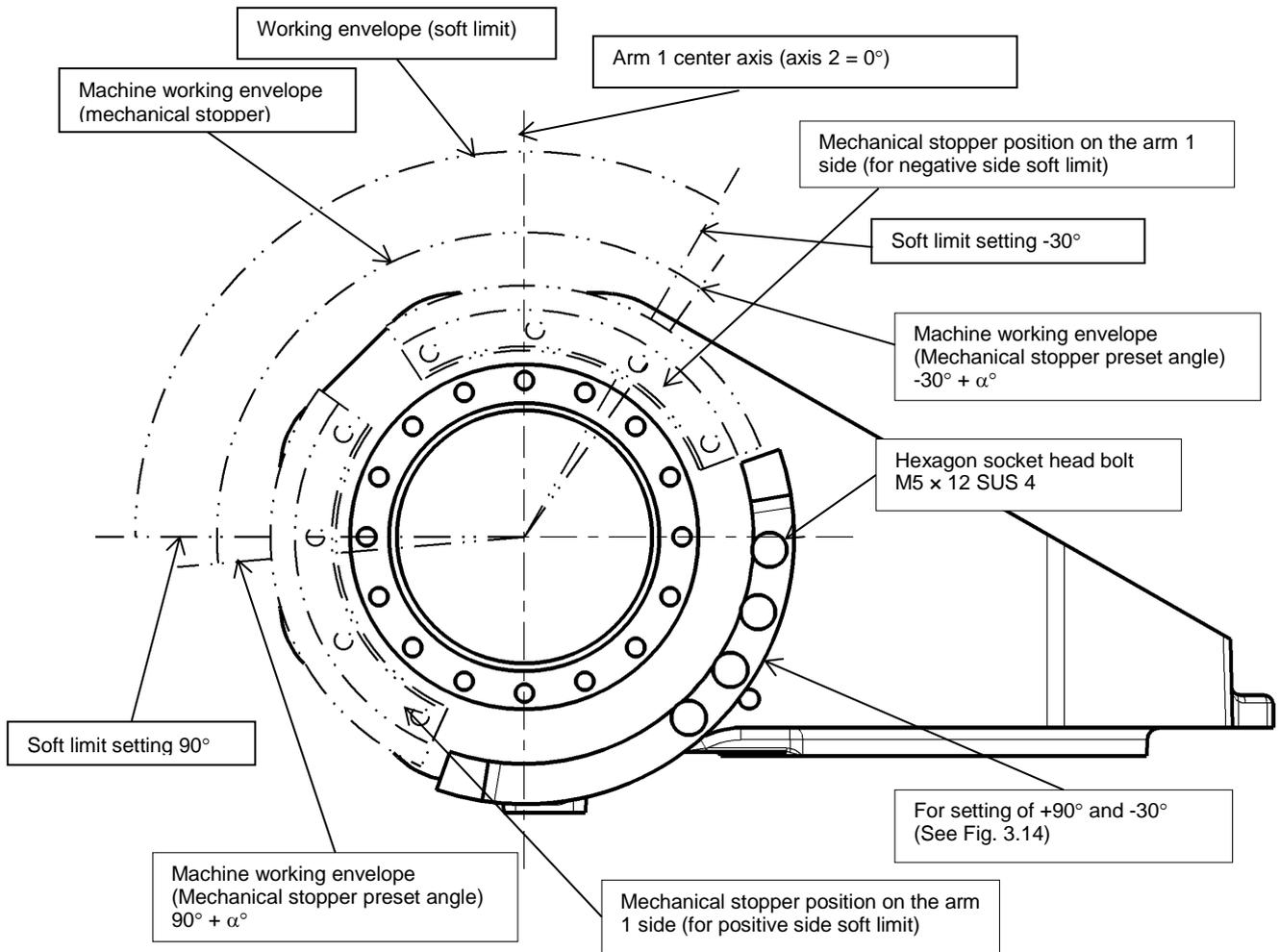
Fig. 3.15 Example of changing axis-2 working envelope (TVL500)
