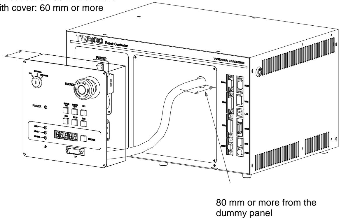
Fig. 9.9 Connection diagram of the dummy panel and the control panel (TS3100)
