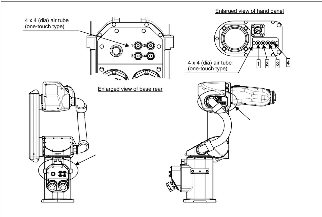
Fig. 10.2 Tool air piping
