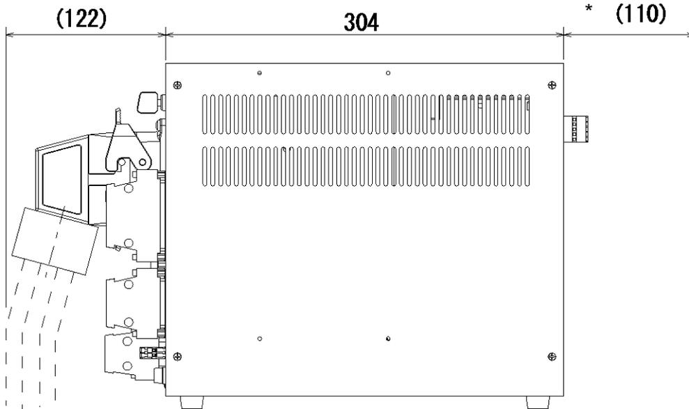
Fig. 4.5 Clearance of controller front side (TSL3100)
