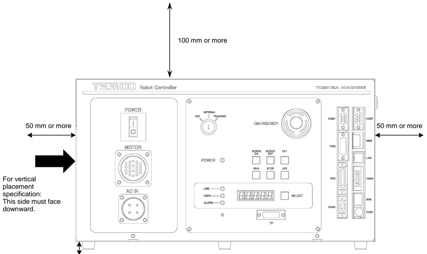
Fig. 6.2 Controller ventilation space
