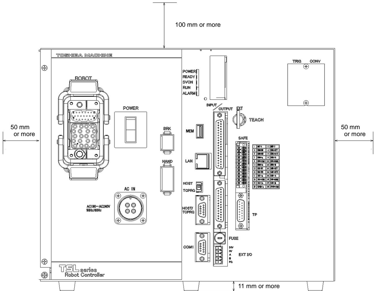
Fig. 5.2 Controller ventilation space (TSL3100E)
