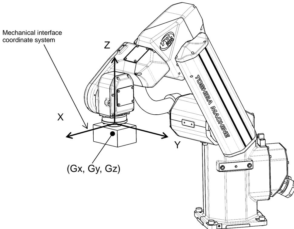
Fig. 10.5 Robot tool coordinate system
