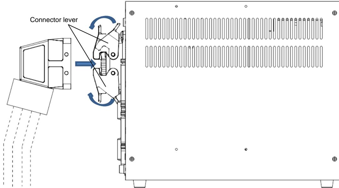
Fig. 7.3 Connecting and disconnecting a ROBOT connector(TSL3100)
