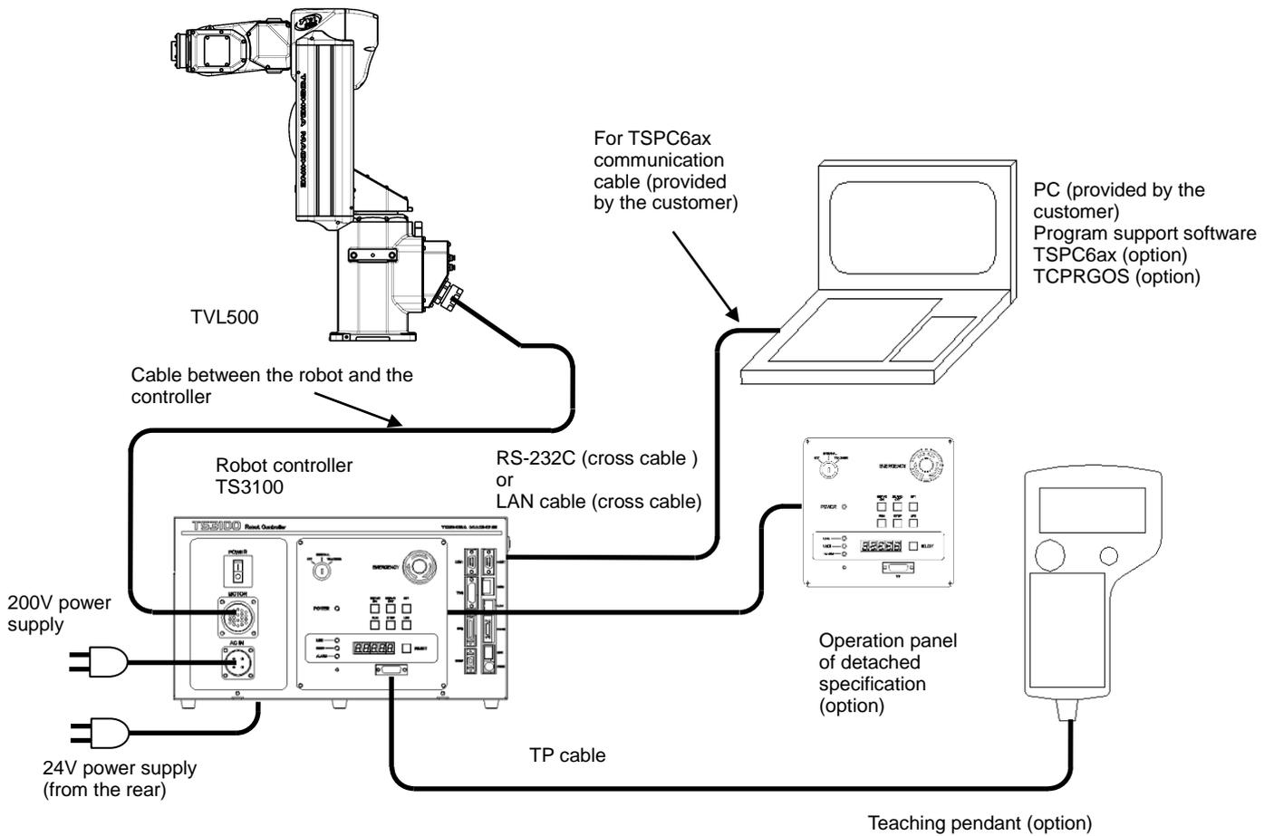
Fig. 1.3 Equipment Configuration (TS3100)
