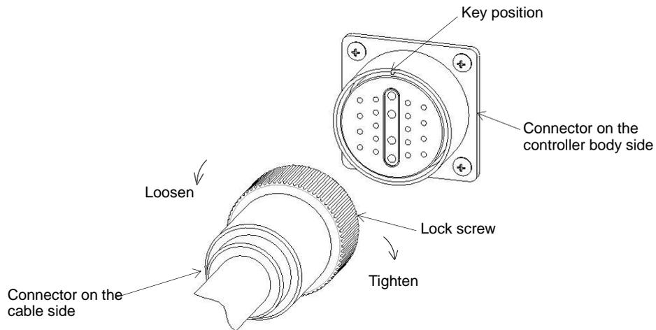
Fig. 9.4 Connecting/disconnecting the circular connector (TS3100)
