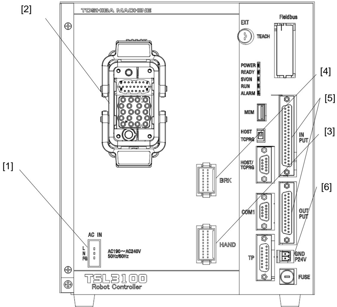
Fig. 7.1 Robot controller connector arrangement (TSL3100)
