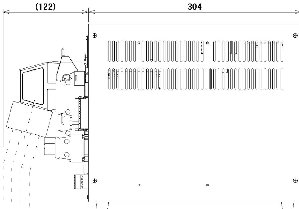
Fig. 5.5 Clearance of controller front side (TSL3100E)
