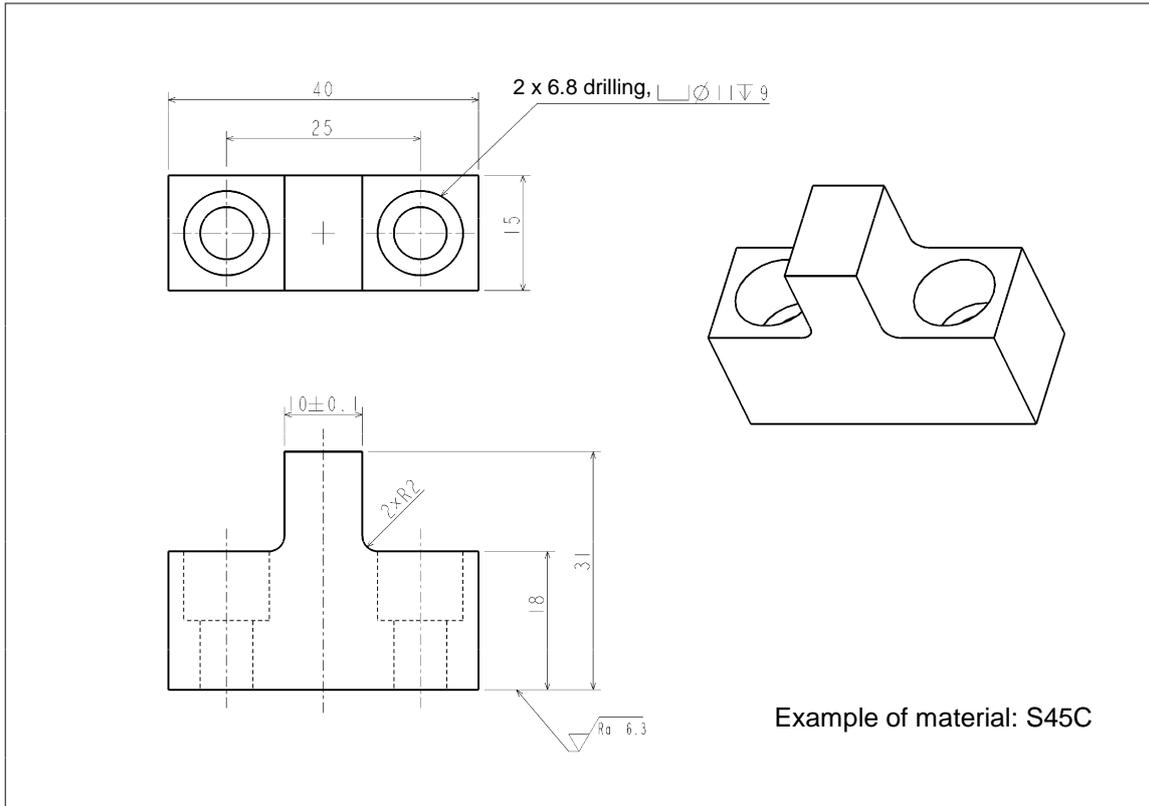
Fig. 3.9 Factory-set mechanical stopper (TVL500/TVL700)
