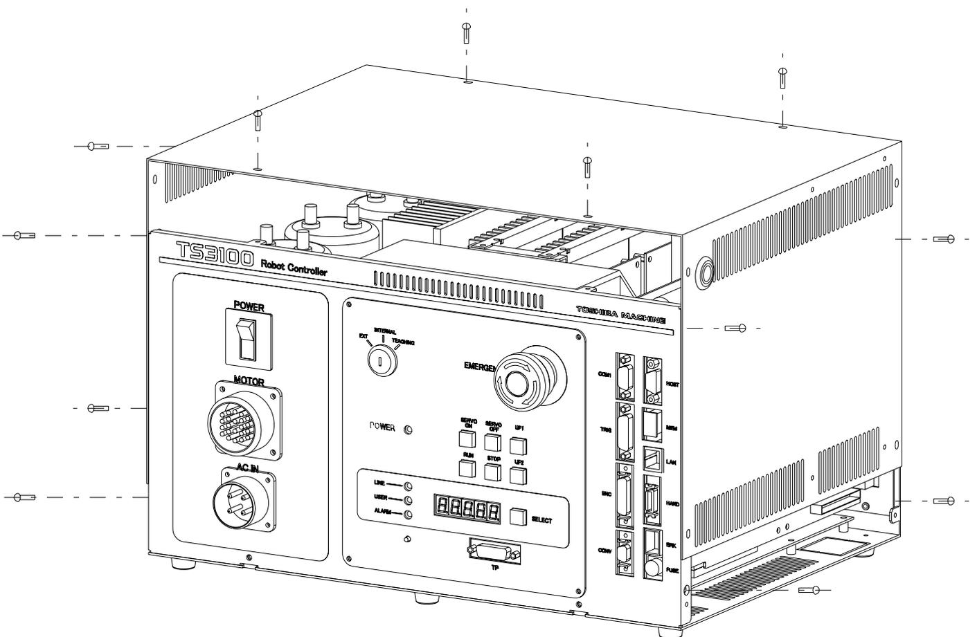
Fig. 1 Removing the TS3000/TS3100 Cover
