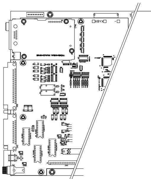
Fig. 7 TSL3000 Robot Controller Side Panel (After Installation of Field Bus Printed Board)
