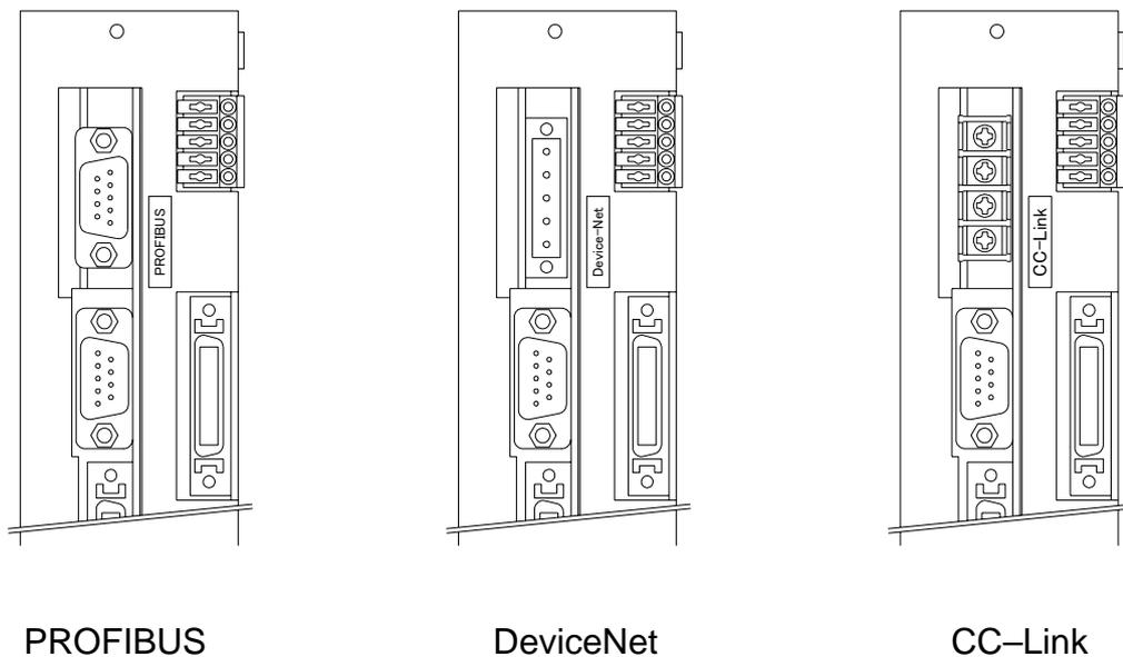
Fig. 4 Rear View of TS3000/TS3100 Controller
