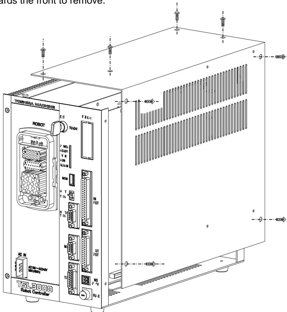
Fig. 5 Removing the TSL3000 Cover
