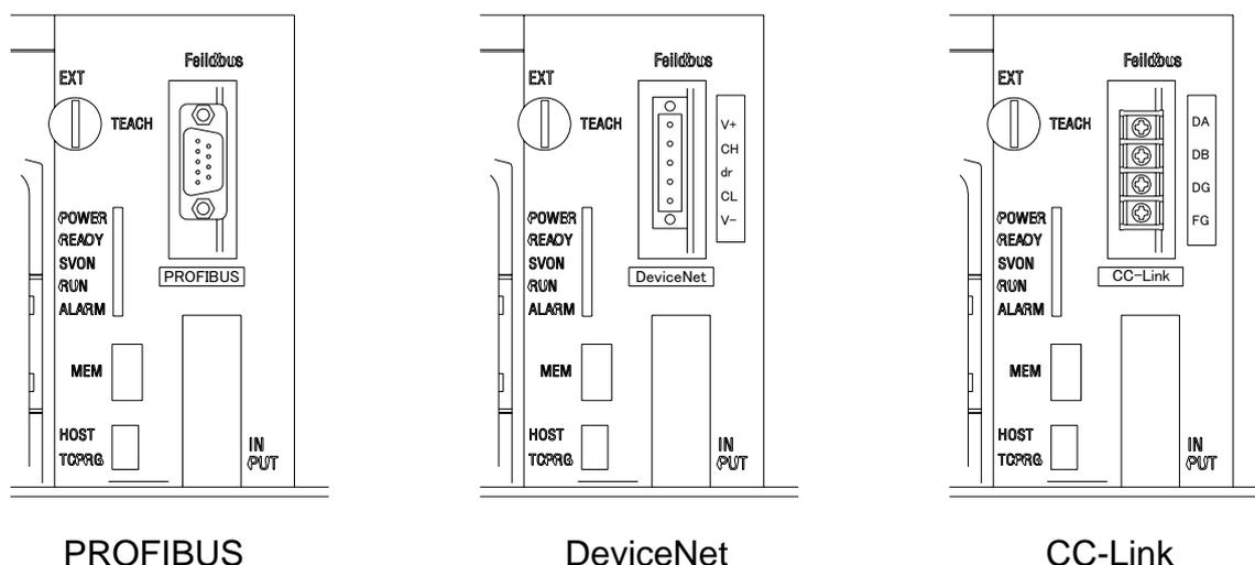
Fig. 8 TSL3000 Controller Front Panel (After Installation of Field Bus Printed Board)
