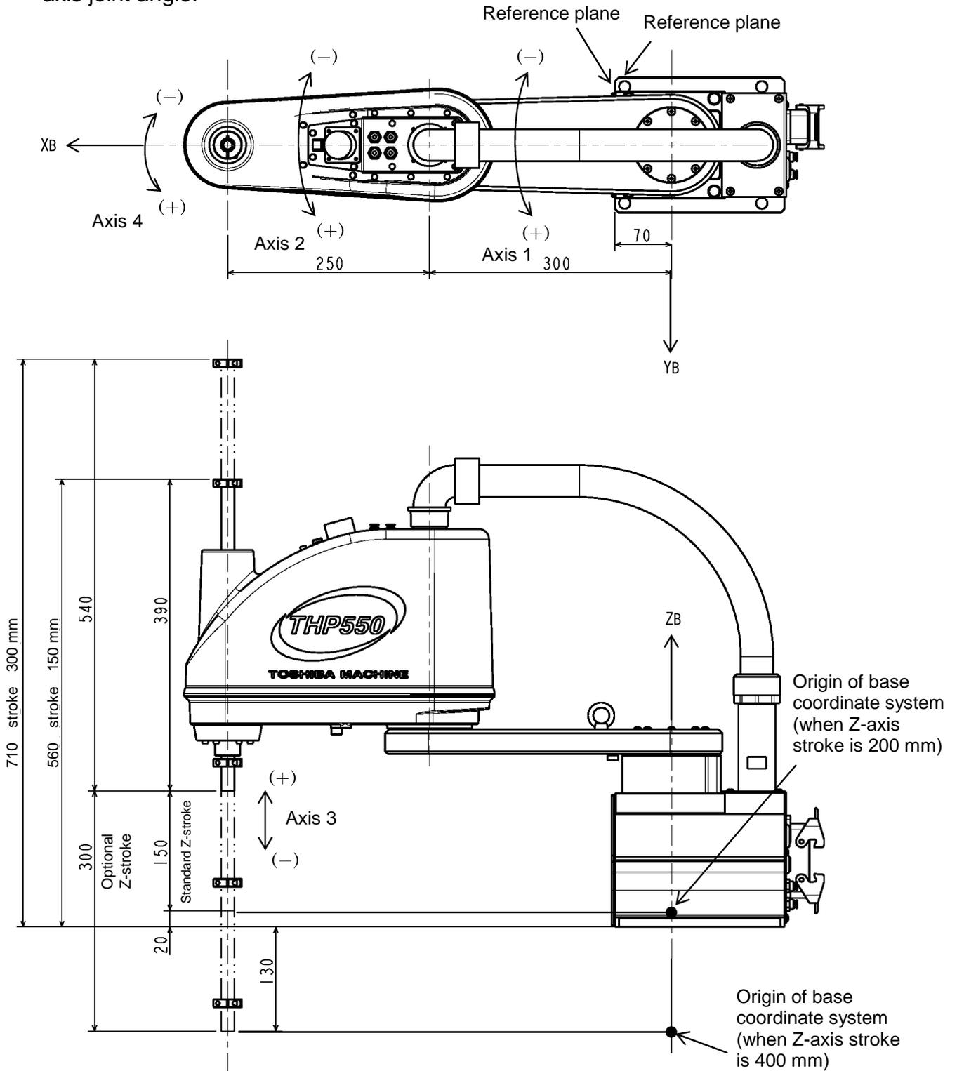
Fig. 3.3 Base coordinate system and joint angle origin
