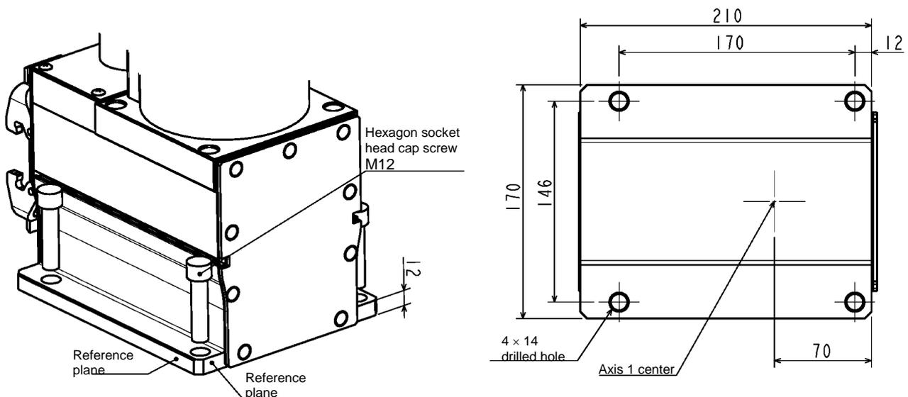
Fig. 3.4 Installation method
