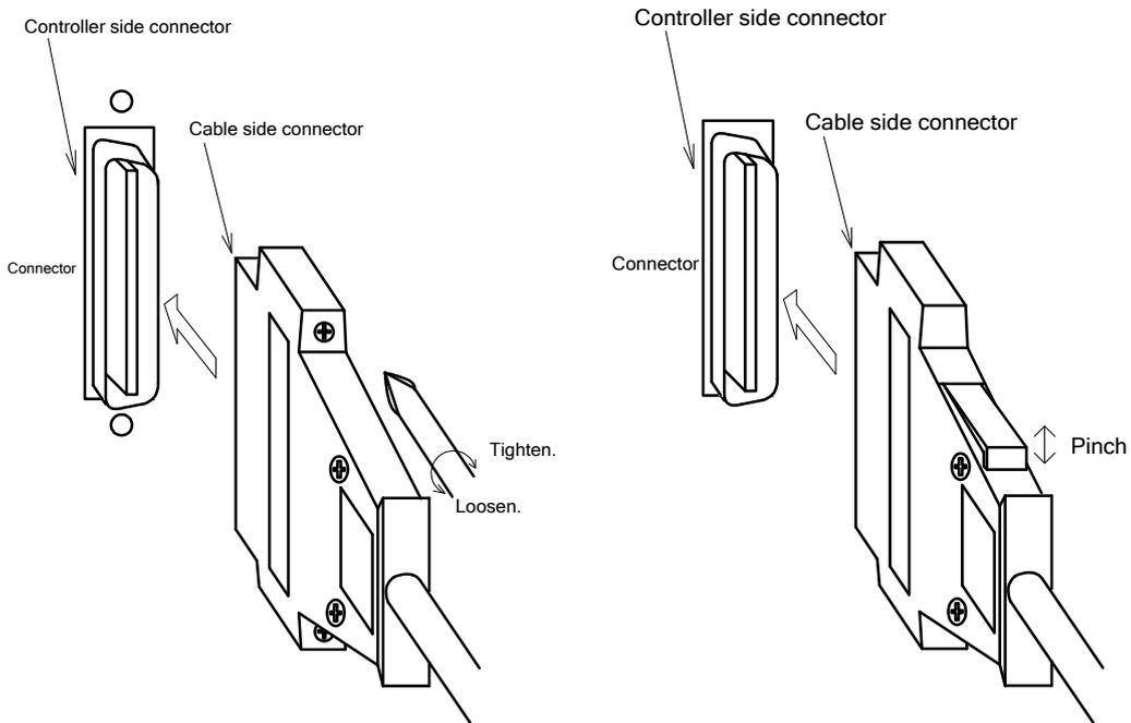
Fig. 4.4 Connecting and disconnecting a square connector
