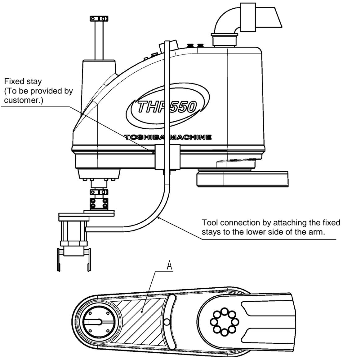
Fig. 5.6 Wiring method ②
