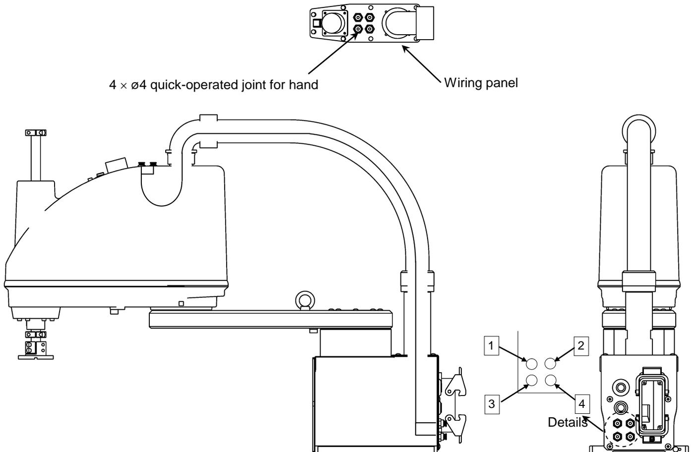
The air tube is identified by the number and color. At piping, make sure that each tube is connected properly, referring to the below-mentioned.
