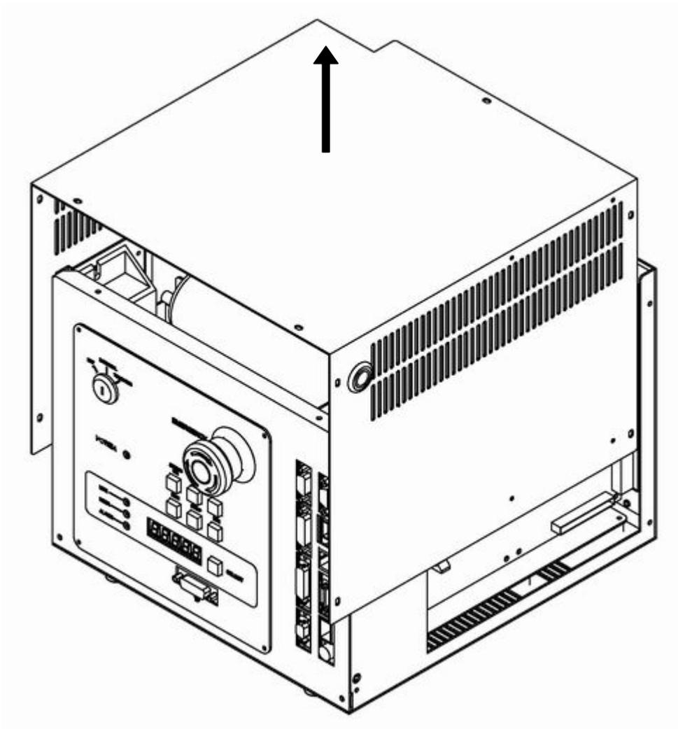
Fig. 3.8 Removing upper cover
