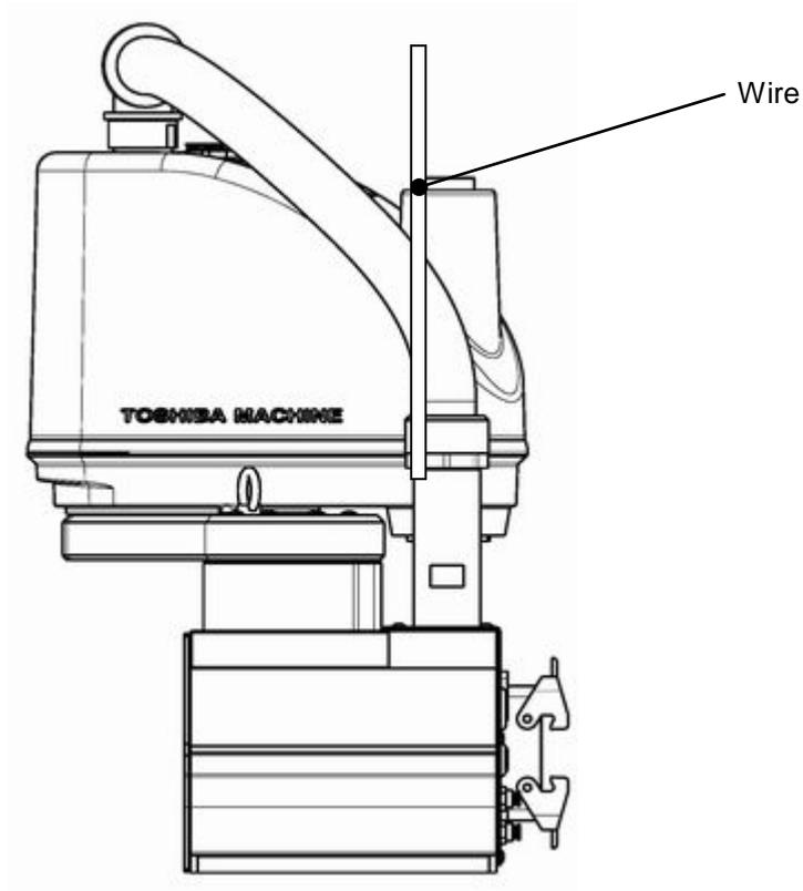
Fig. 2.3 Lifting up the robot
