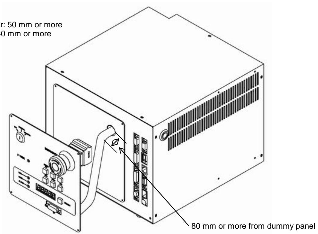
Fig. 4.8 Cable connections of dummy panel and control panel
