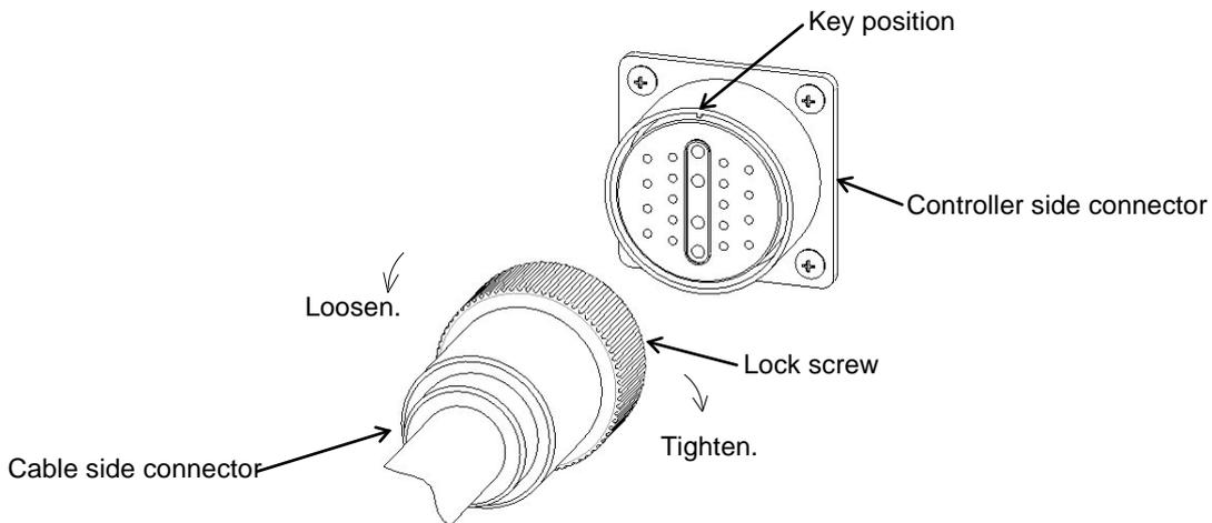
Fig. 4.3 Connecting and disconnecting a circular connector
