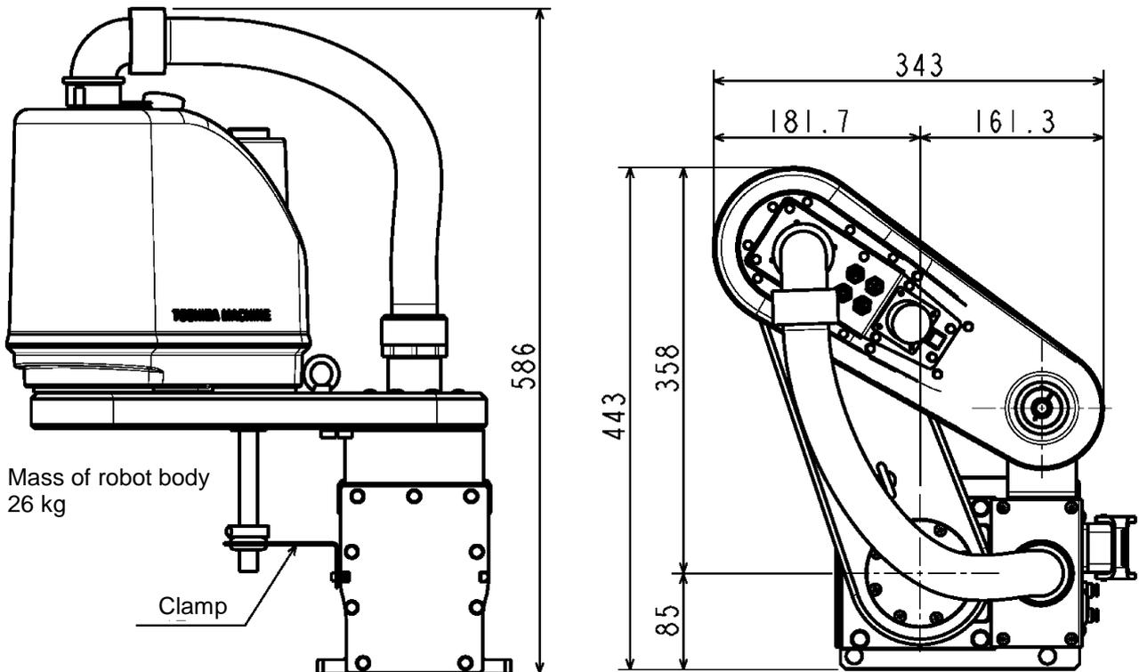
Fig. 2.2 Outer dimensions at transport (THP550)
