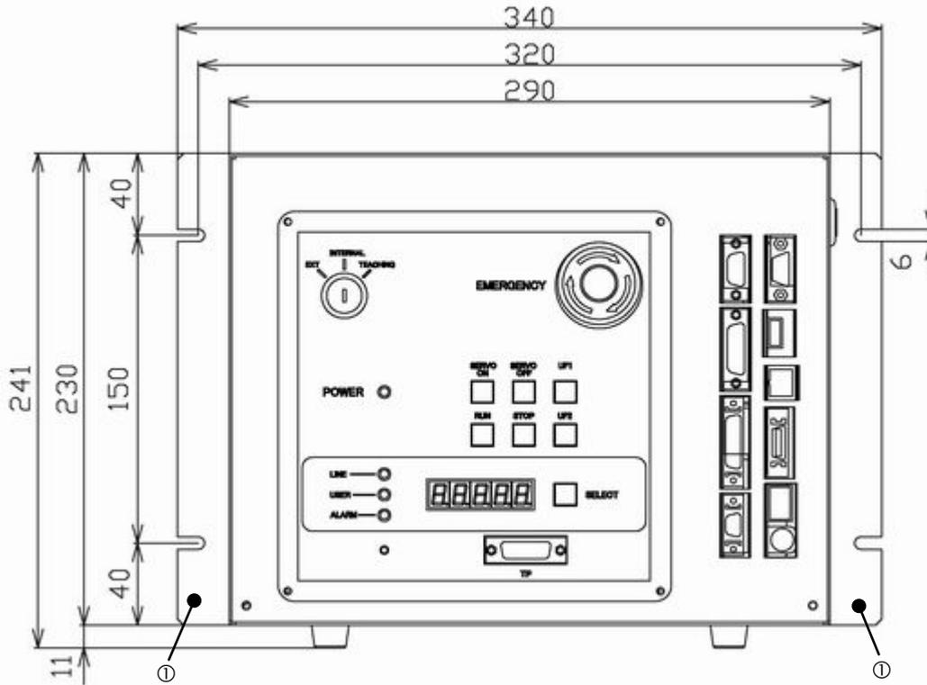
Fig. 3.7 Screw hole dimensions for securing controller
