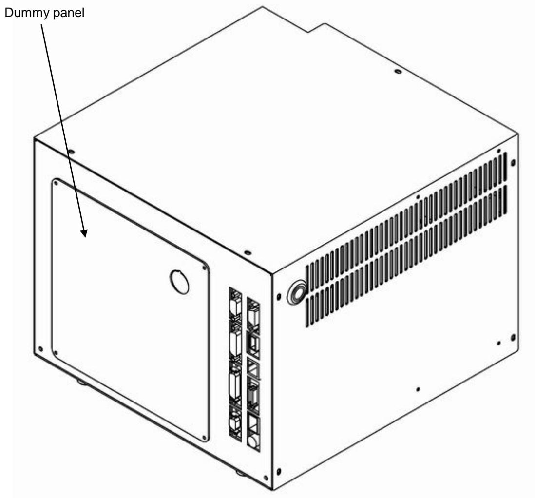
Fig. 4.7 Mounting dummy panel
