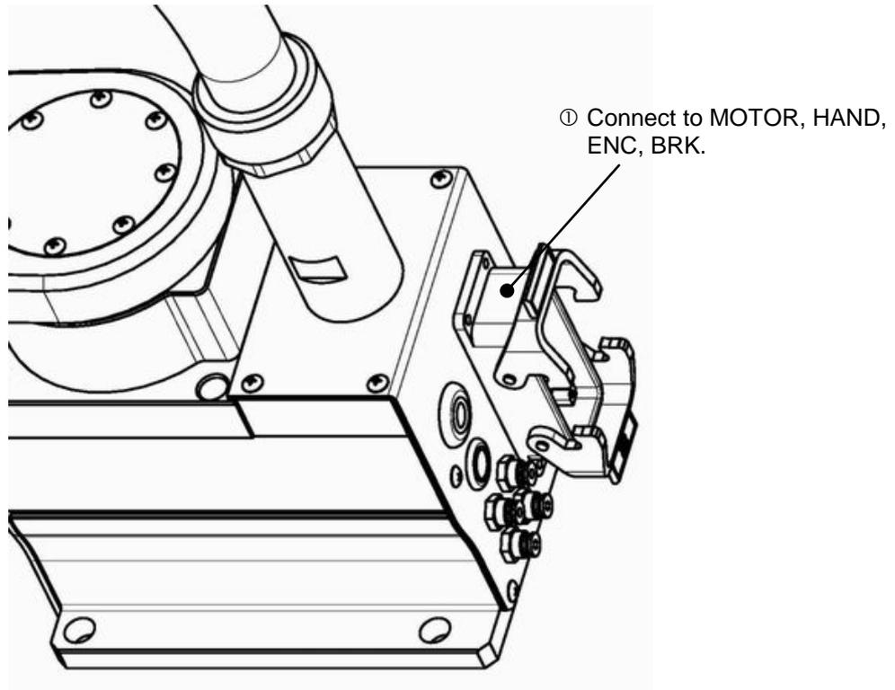
Fig. 4.2 Robot side connector arrangement
