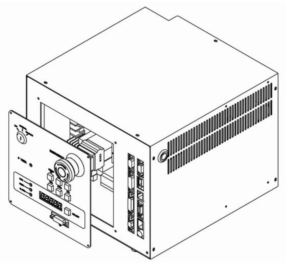
Fig. 4.5 Removing control panel
