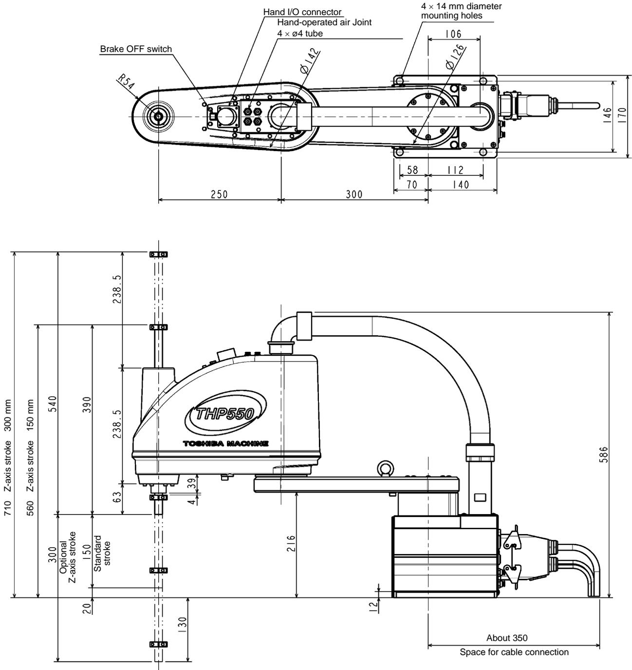
Fig. 1.3 External dimensions of the robot (THP550)
