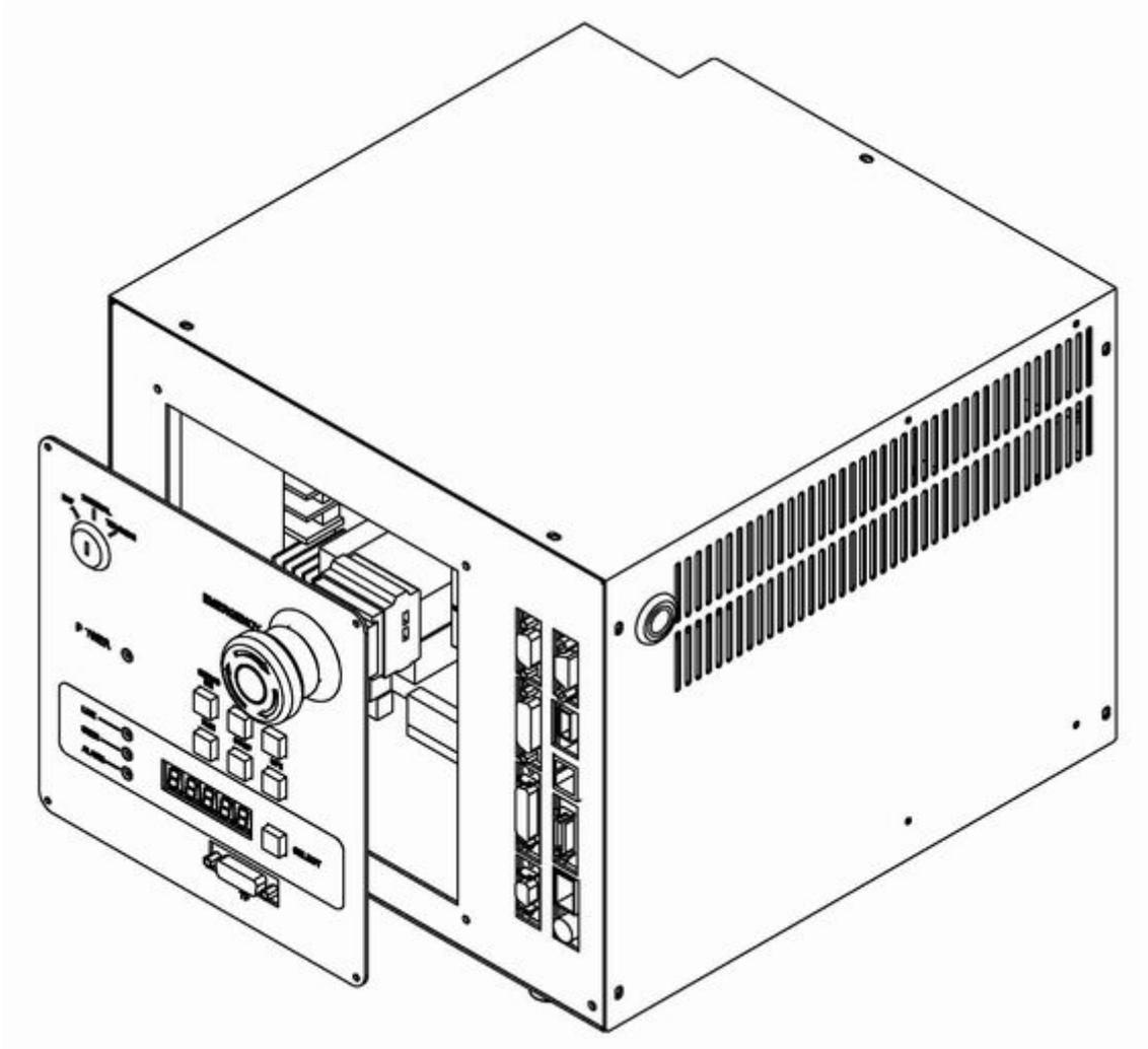
**Fig. 3.7 Removing control panel**
