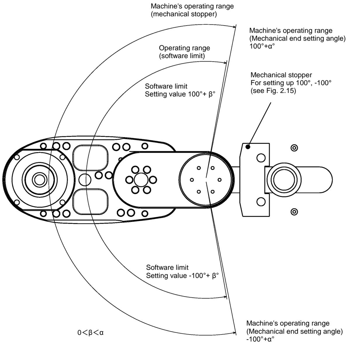
Fig. 2.16 Example of changing the mechanical ends of Axis 1
