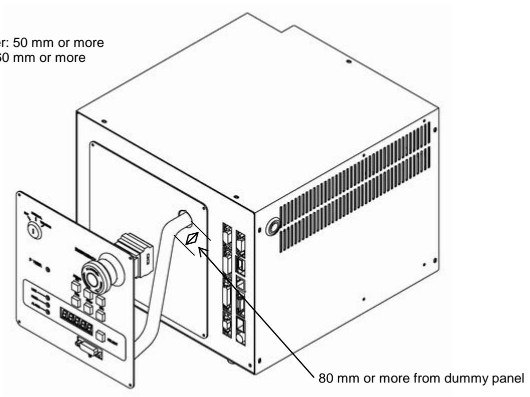
**Fig. 3.10 Cable connections of dummy panel and control panel**
