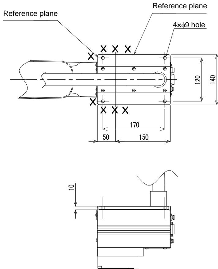
Fig. 2.11 Installing the TH350A- T robot
