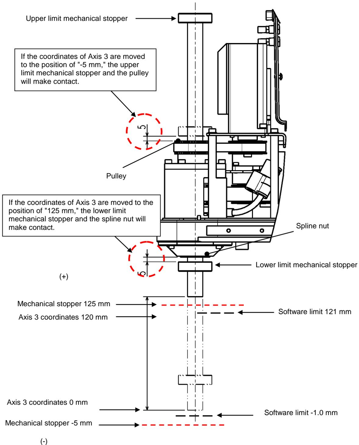
Fig. 2.19 Axis 3 mechanical end settings
