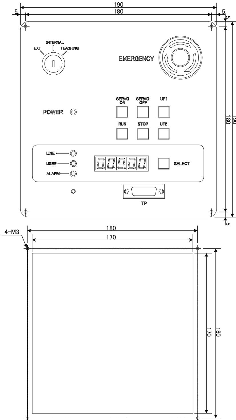
**Fig. 3.8 Control panel mounting dimensions**
