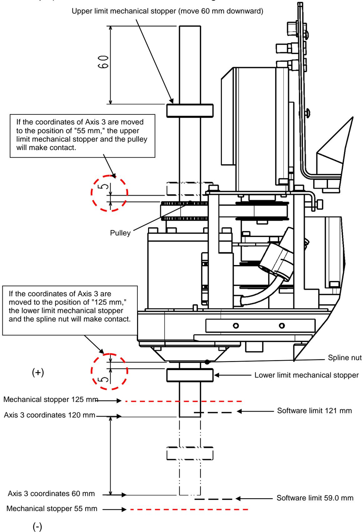
Fig. 2.23 Example of changing the mechanical ends of Axis 3
