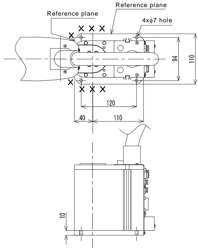
Fig. 2.10 Installing the TH180 robot
