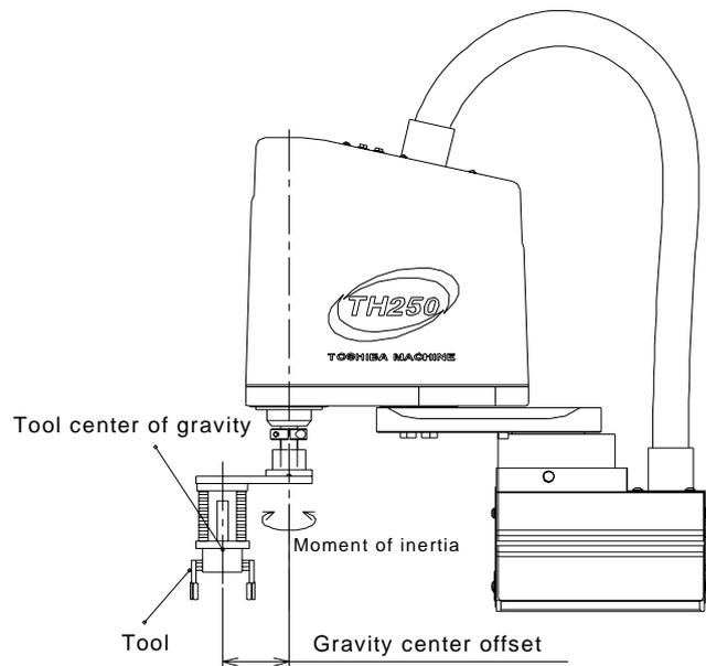
Fig. 4.6 Tool and robot body (Normal type)
