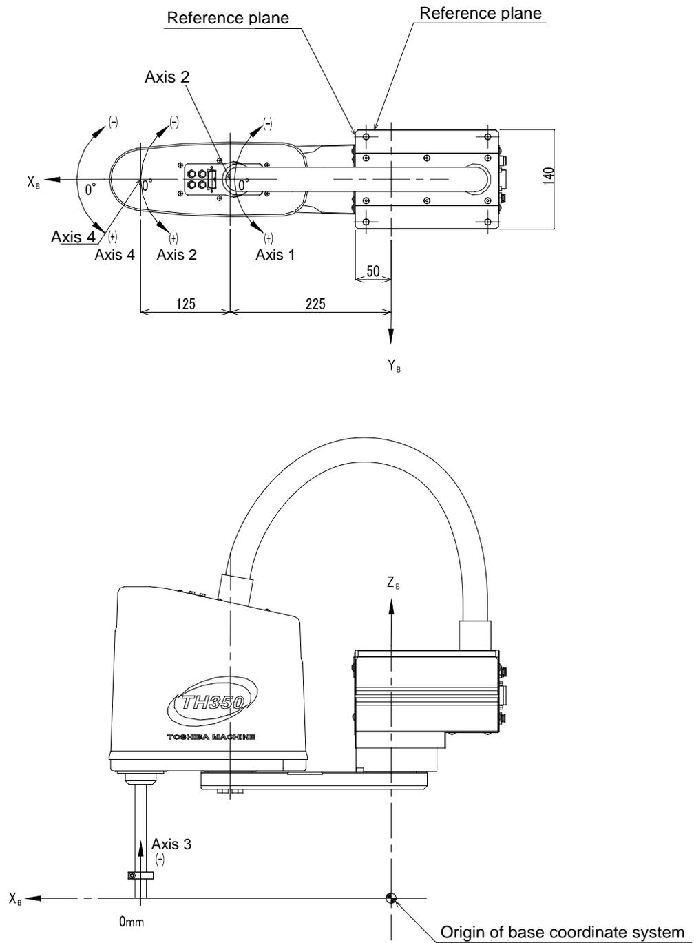
Fig. 2.8 TH350A- T base coordinate system and joint angle origin
