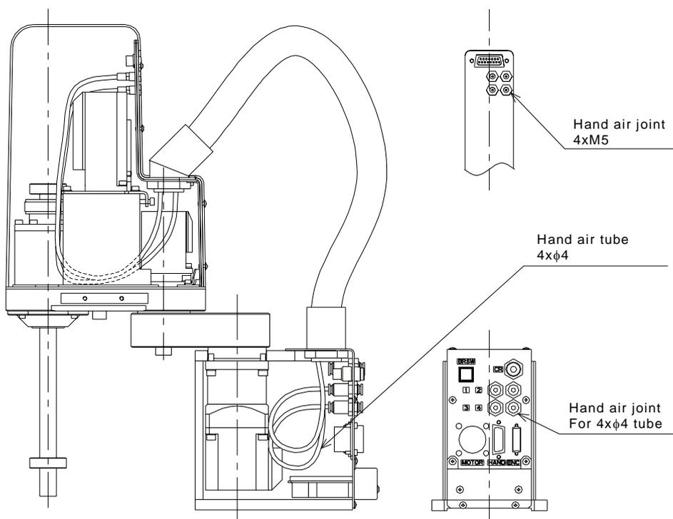
Fig. 4.4 Air piping for tool (TH180)
