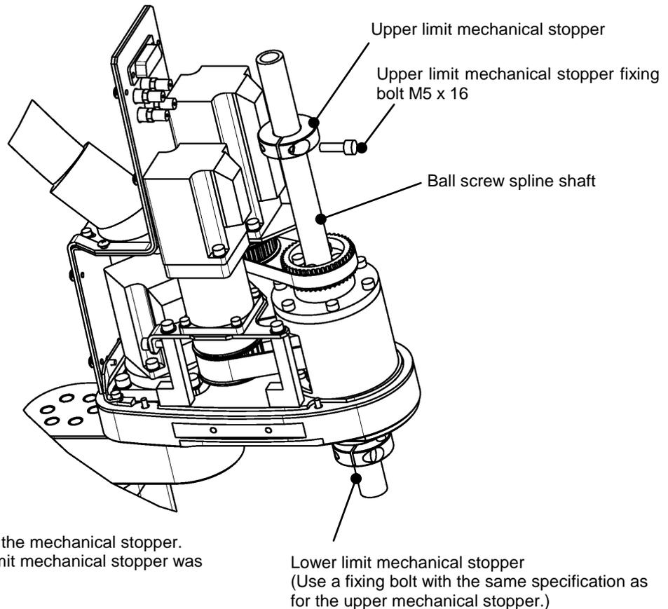
Change the fixing position of the mechanical stopper.
