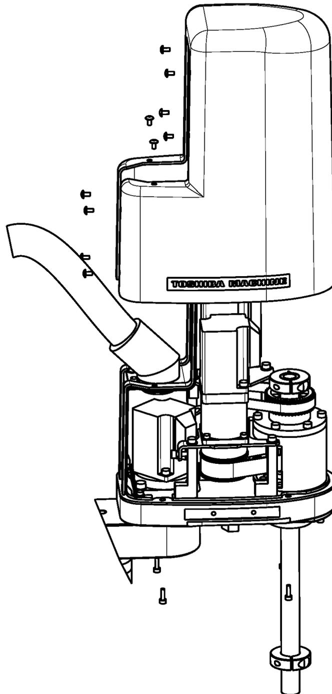
Fig. 2.20 Removing the Arm 2 cover
