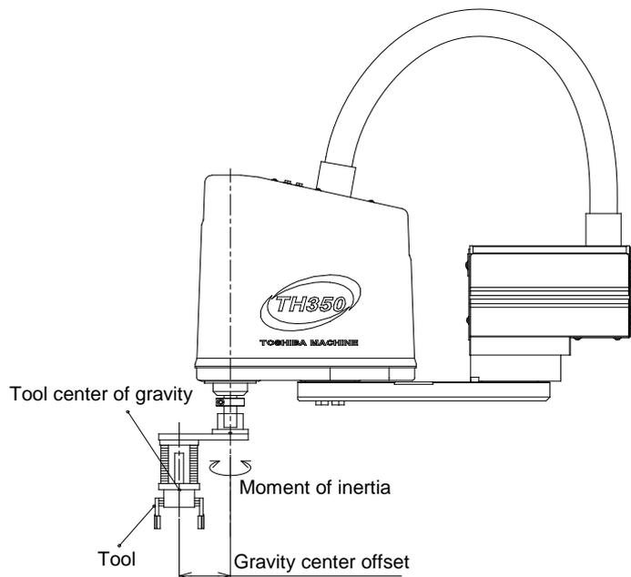
Fig. 4.7 Tool and robot body (Ceiling type)
