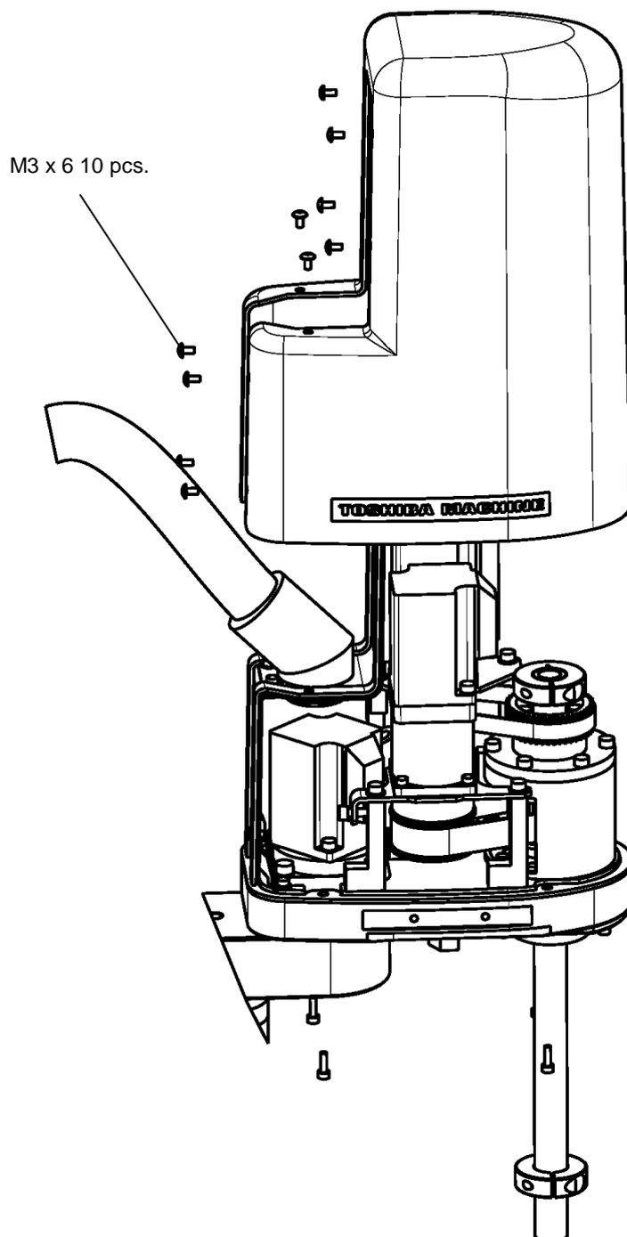
Fig. 2.24 Reinstalling the Arm 2 cover
