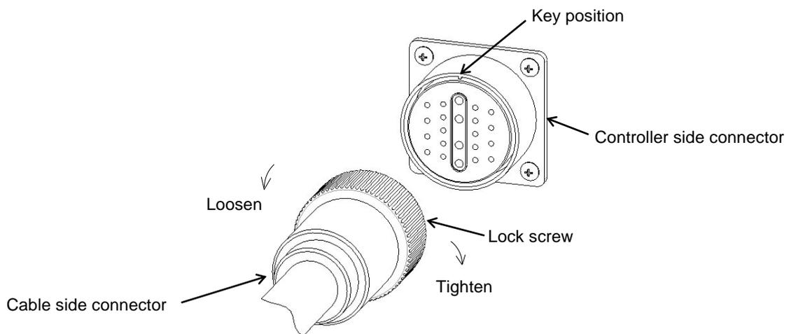
Fig. 3.5 Inserting and removing a circular connector
