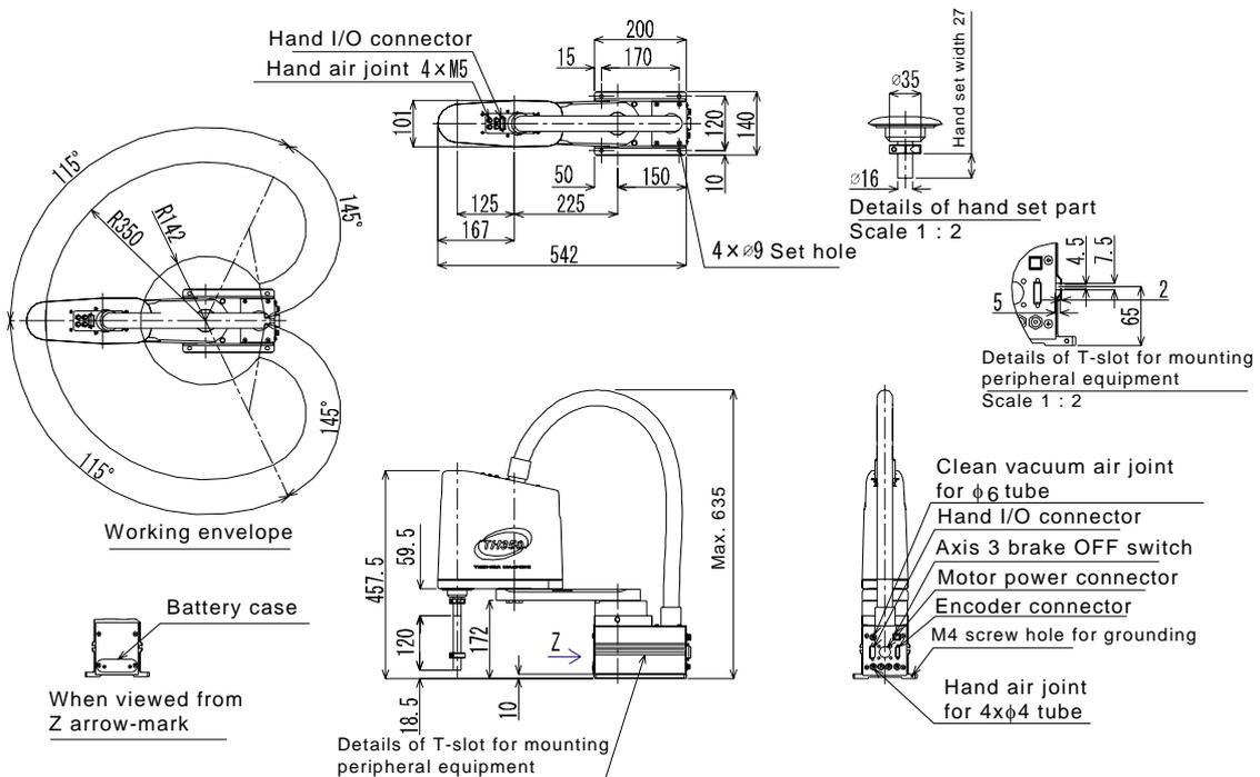
Fig. 2.2 External view of TH350A robot
