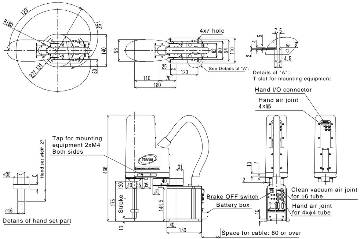
Fig. 2.3 External view of TH180 robot
