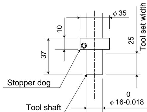
(a) Dimensions of tool shaft section
