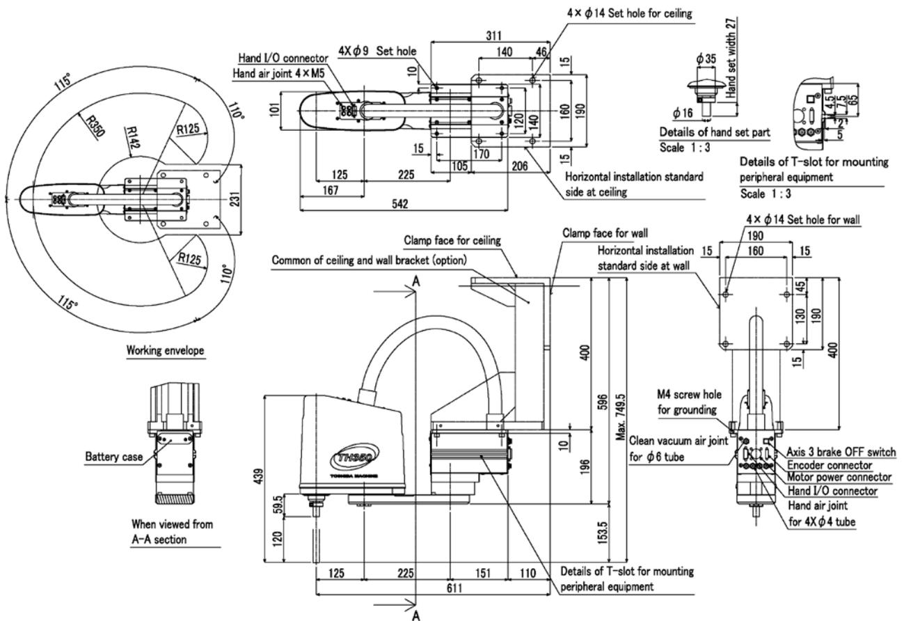
Fig. 2.4 External view of TH350A- T robot
