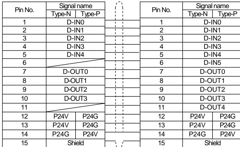
Fig. 4.2 Machine I/O harness wiring
