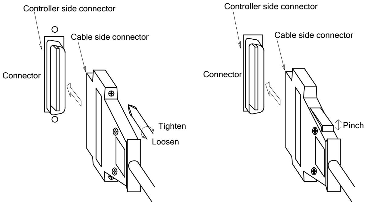
Fig. 3.6 Inserting and removing a square connector
