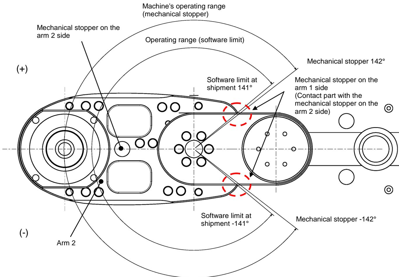
Fig. 2.13 Axis 2 mechanical end settings (TH180)
