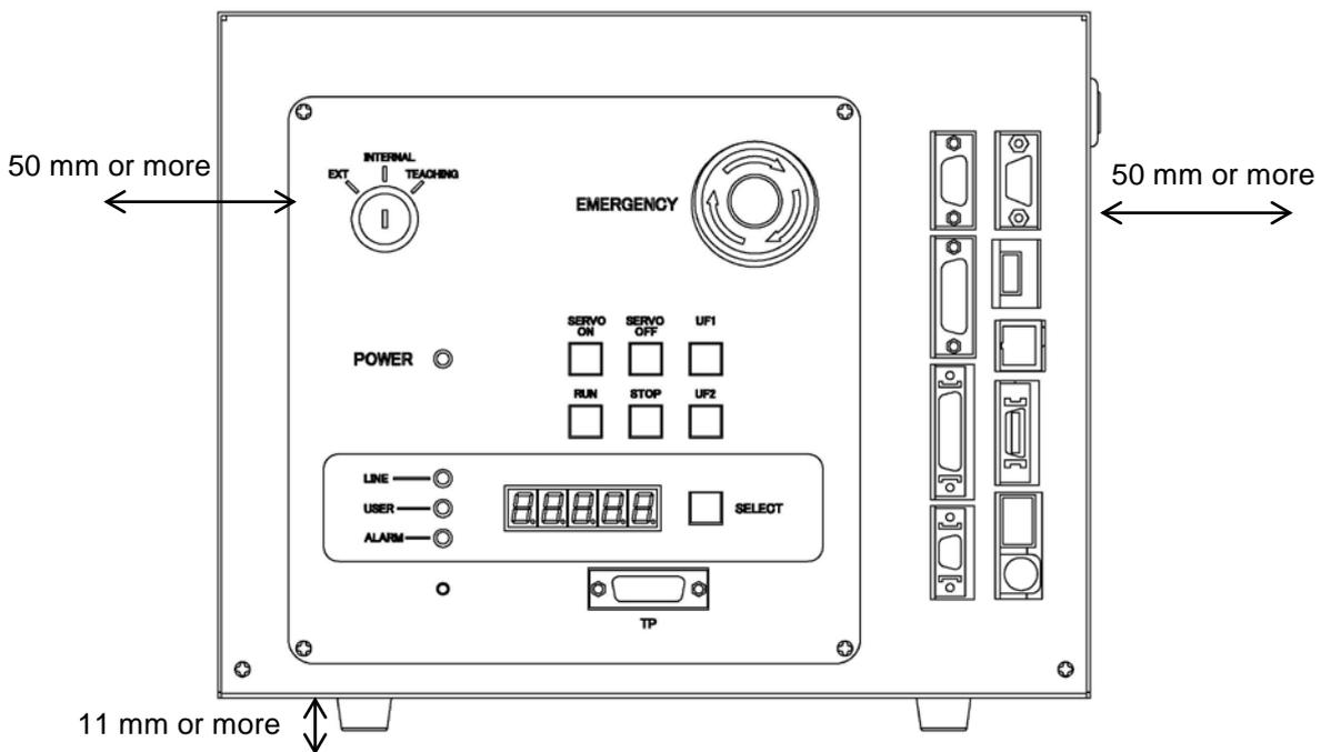
Fig. 2.26 Spaces for ventilating the controller
