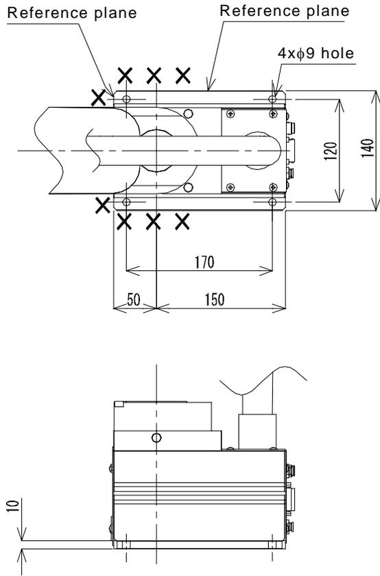
Fig. 2.9 Installing the TH250A and TH350A robots
