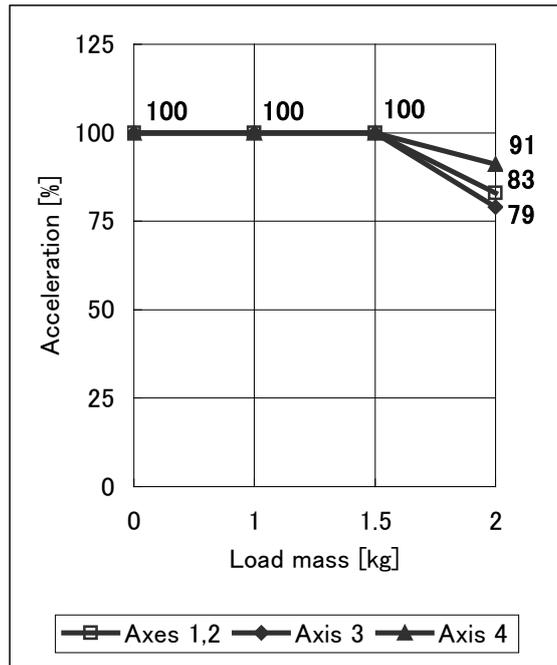
Fig. 4.14 Setting of acceleration for load mass (TH180)
