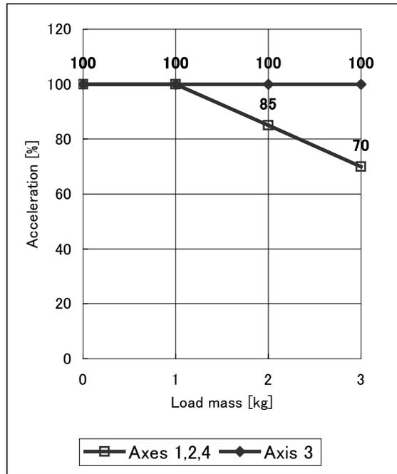
Fig. 4.12 Setting of acceleration for load mass (TH350A)
