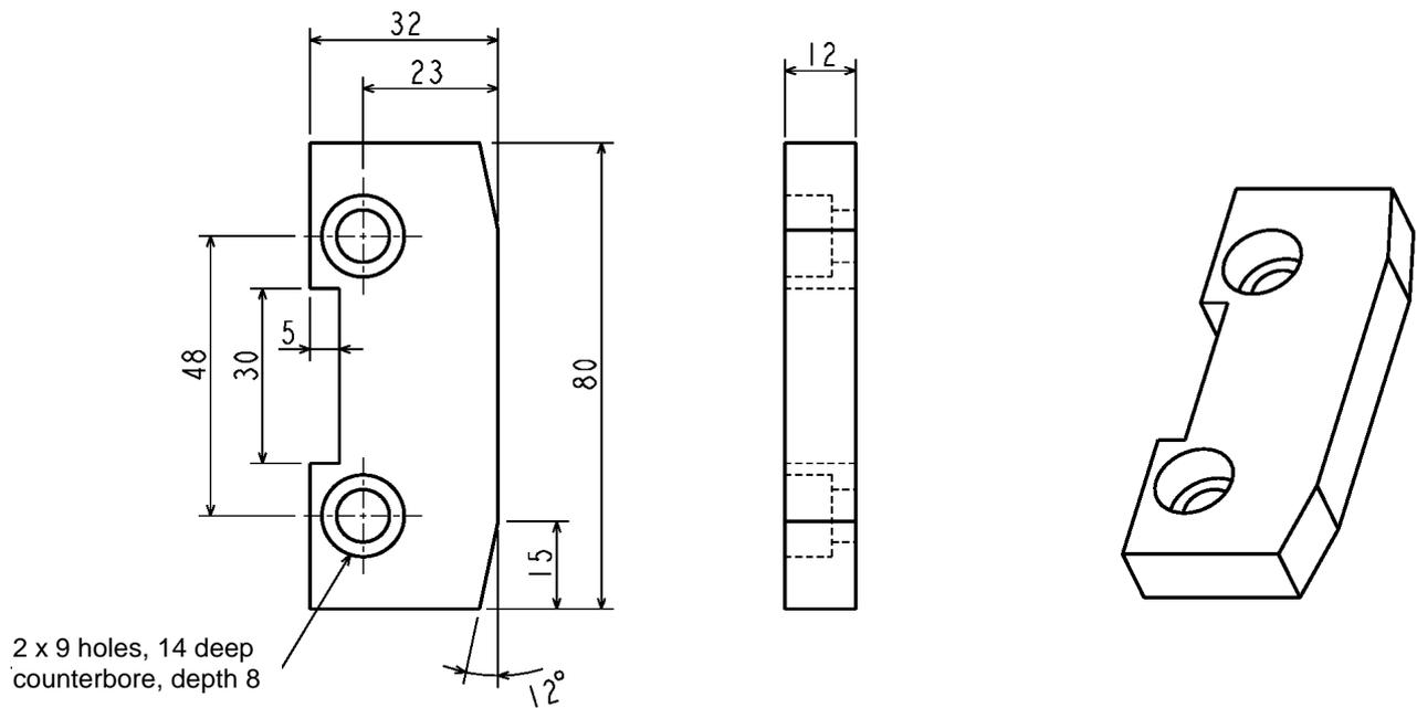
Fig. 2.15 Example of changing the mechanical stopper for Axis 1
