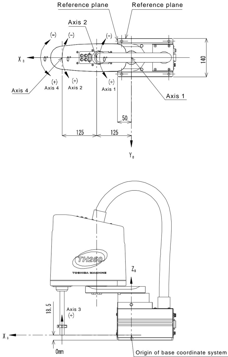
Fig. 2.6 TH350A base coordinate system and joint angle origin
