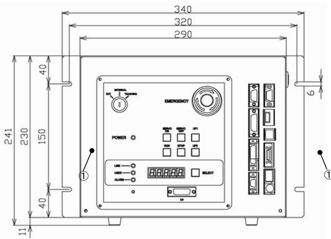
Fig. 2.27 Screw hole dimensions for securing controller
