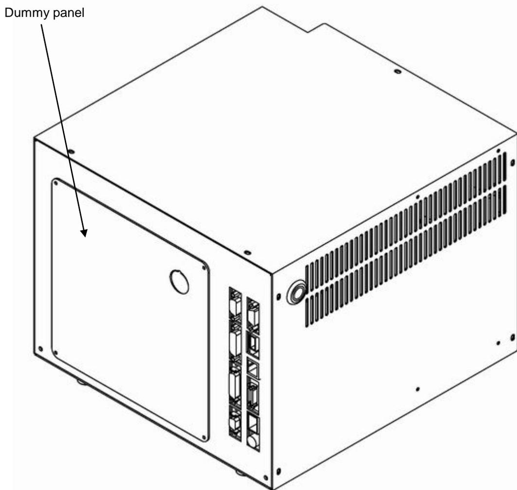
**Fig. 3.9 Mounting dummy panel**
