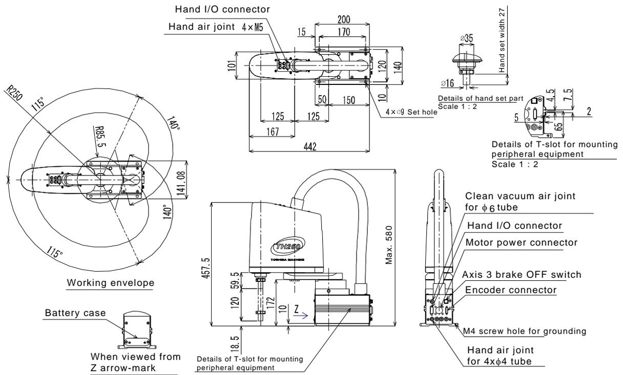
Fig. 2.1 External view of TH250A robot
