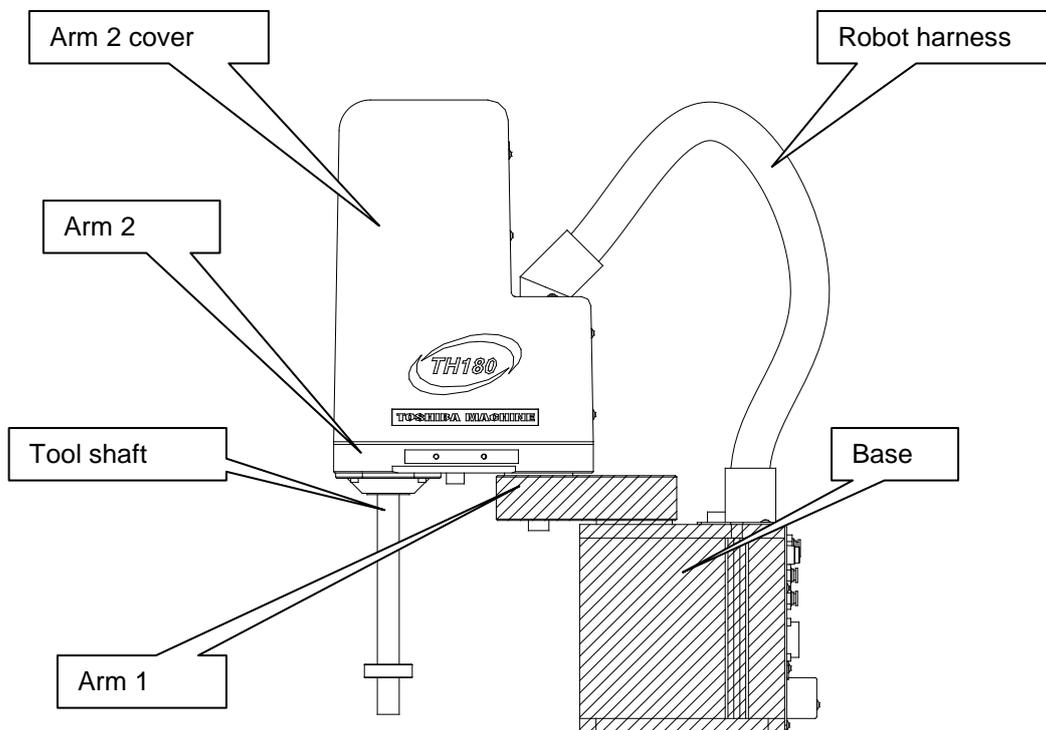
Fig. 1.5 Robot handling area (shaded area) (TH180)
