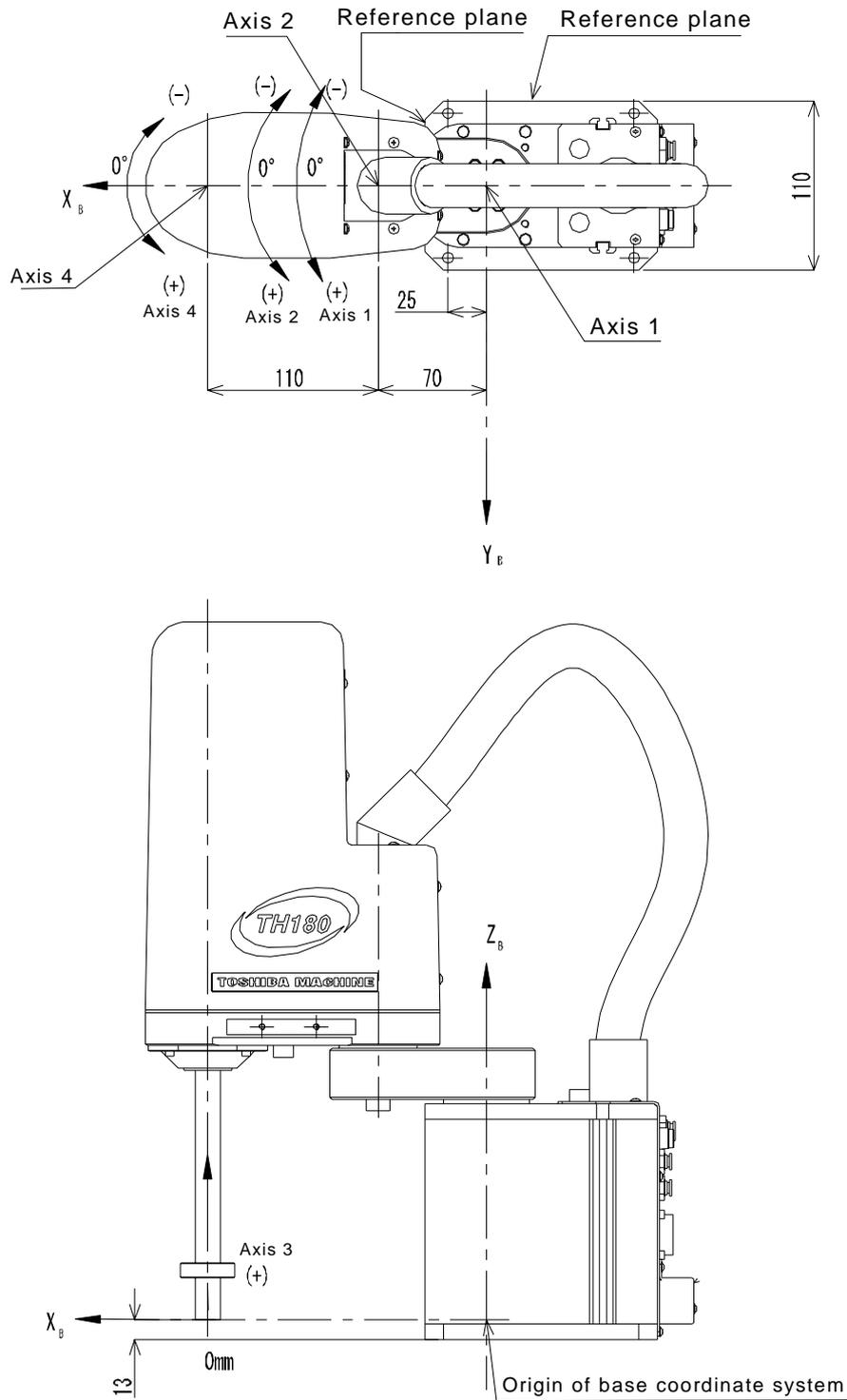
Fig. 2.7 TH180 base coordinate system and joint angle origin
