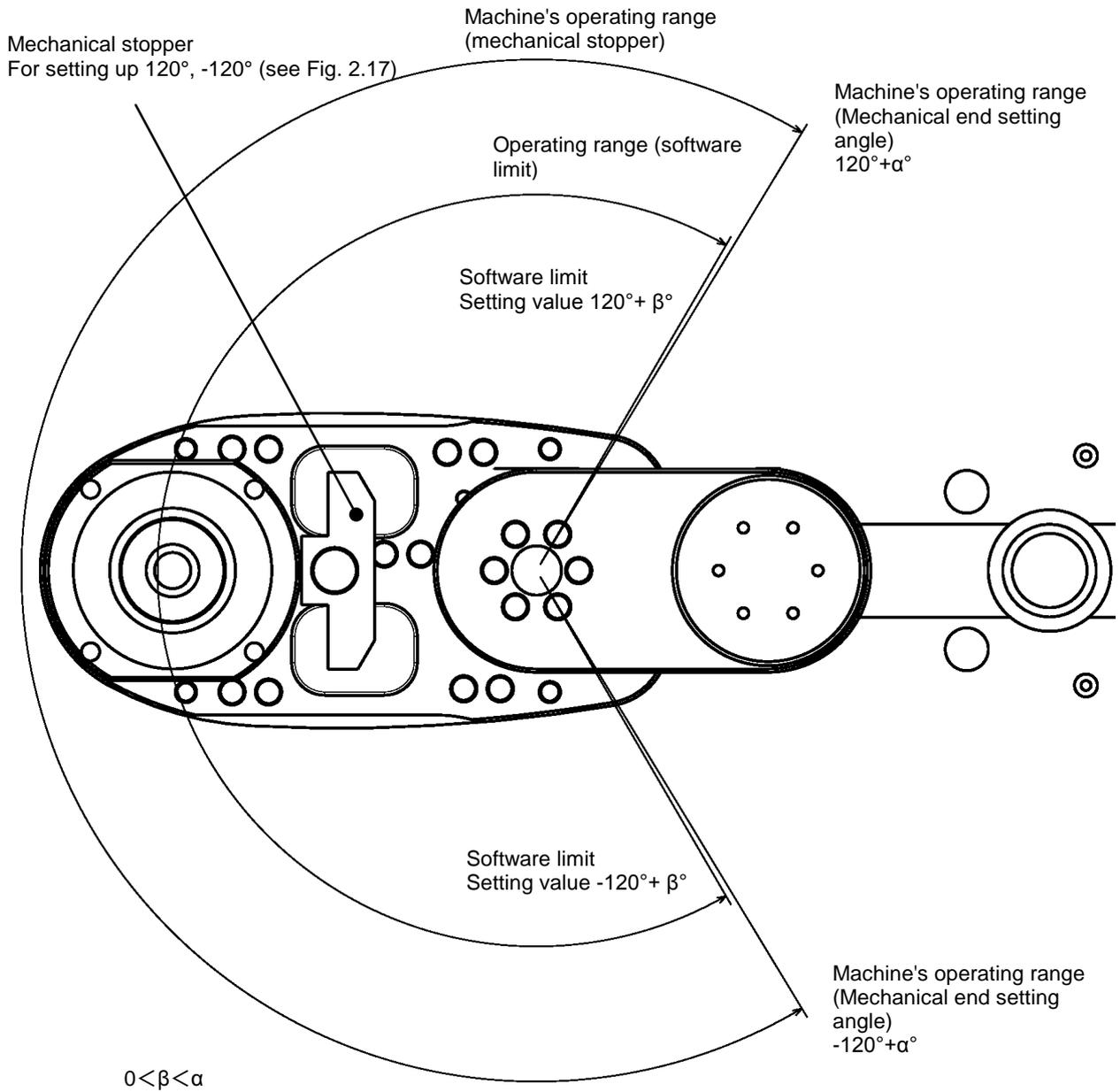
Fig. 2.18 Example of changing the mechanical ends of Axis 2
