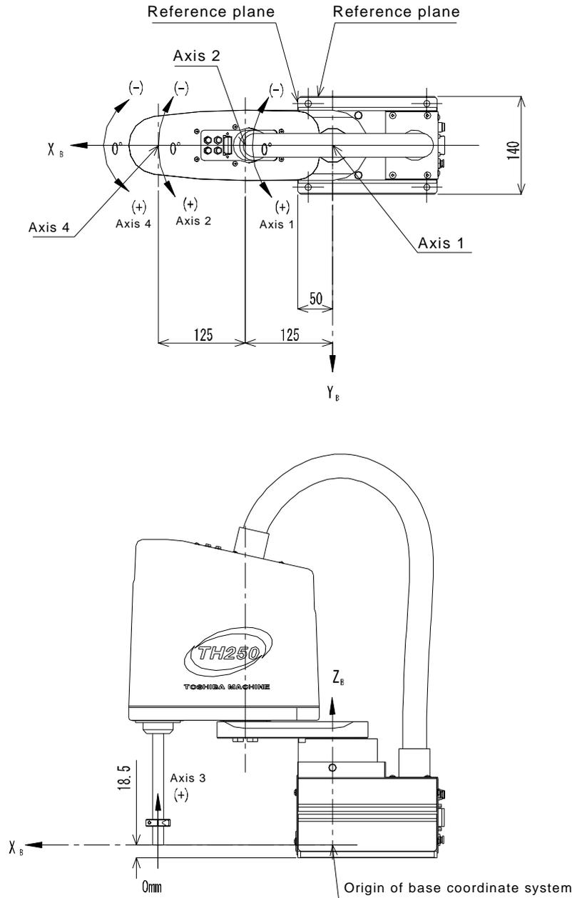
Fig. 2.5 TH250A base coordinate system and joint angle origin
