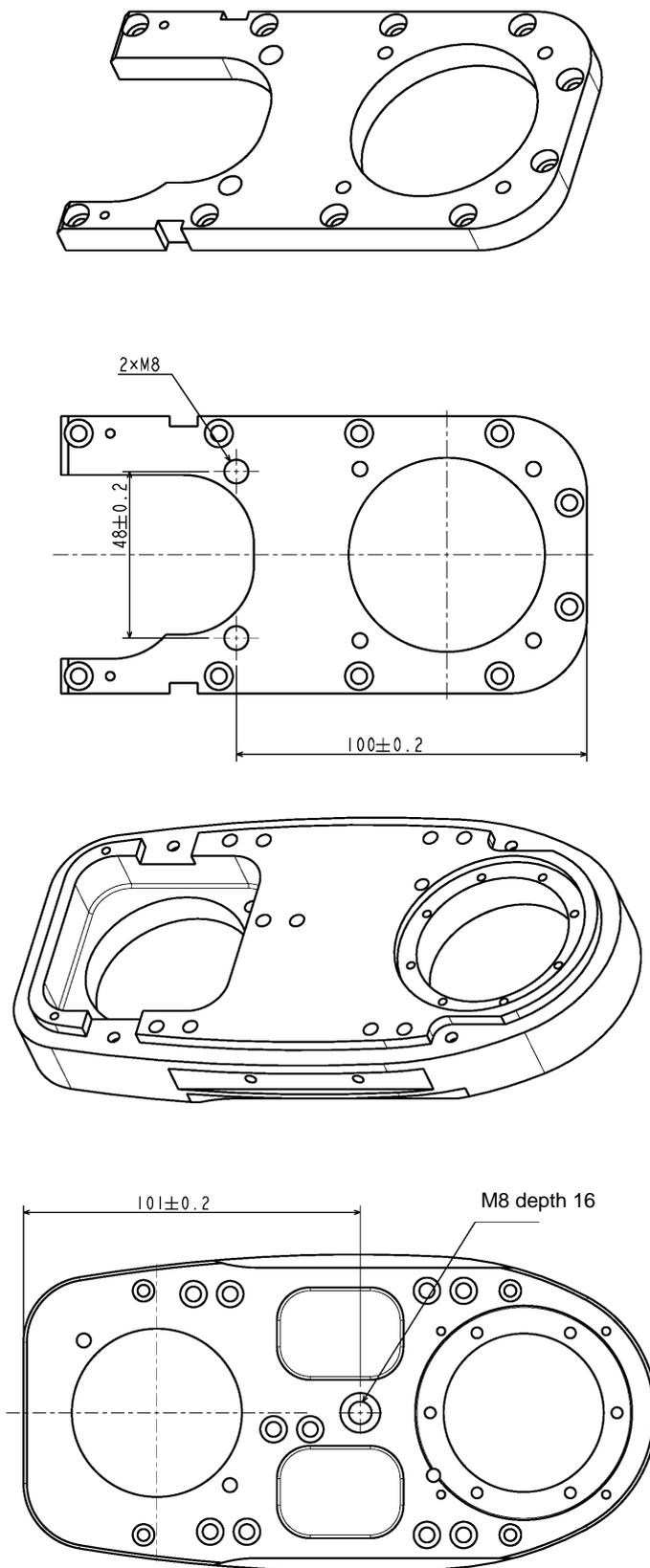
Fig. 2.14 Mechanical stopper installation positions
