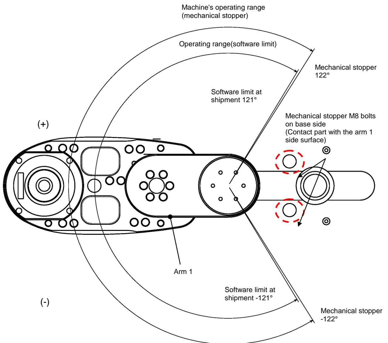
Fig. 2.12 Axis 1 mechanical end settings (TH180)
