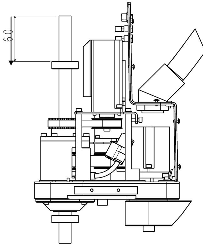
Fig. 2.21 Moving the mechanical stopper
