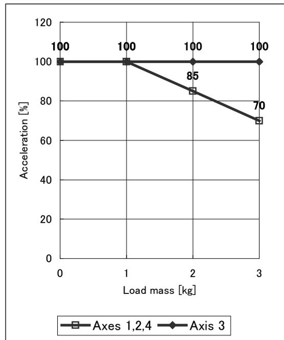
Fig. 4.16 Setting of acceleration for load mass (TH350A)
