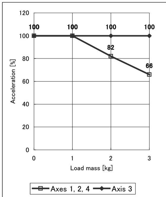
Fig. 4.8 Setting of acceleration for load mass (TH250A)
