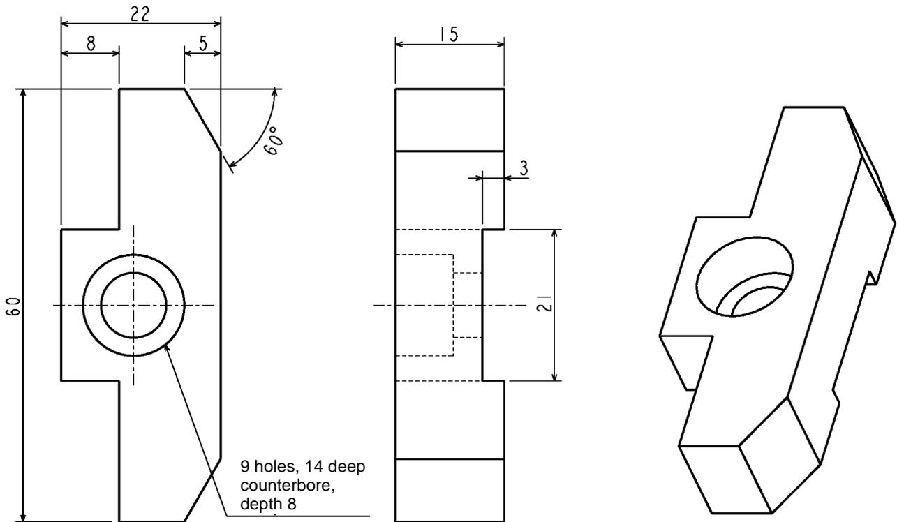
Fig. 2.17 Example of changing the mechanical stopper for Axis 2
