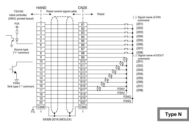
[Type N] (When X8GN printed board is used)
