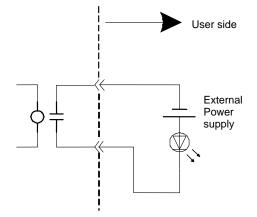
\* The above figure exemplifies a normal open contact output structure.
