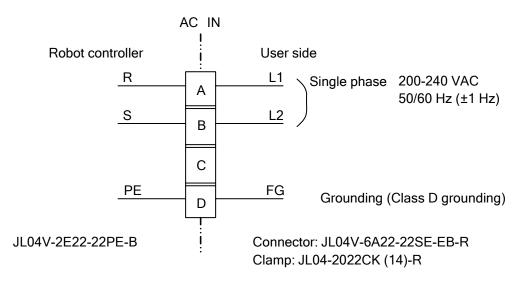
Fig. 1 Connection of power cable
