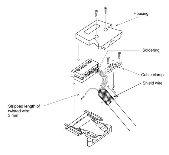
Note: The shield wire of the robot control signal cable is connected to the ground of the TS3100 robot controller through the housing. Completely connect the shield wire to the housing using the cable clamp.
