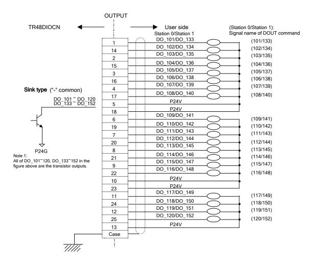
The specifications of the extension output signal are the same as those of the digital output signal (i.e., sink type) which are described in Para. 4.8.
