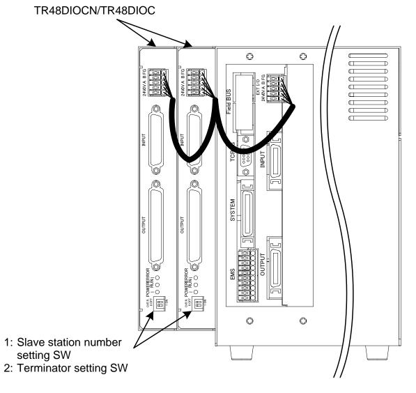
Fig. 7.4 Connection of TR48DIOCN/TR48DIOC module
