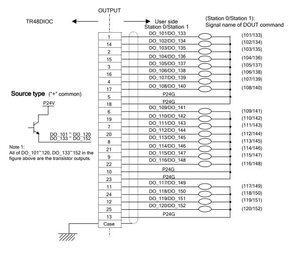
The specifications of the extension output signal are the same as those of the digital output signal (i.e., source type) which are described in Para. 4.8.
