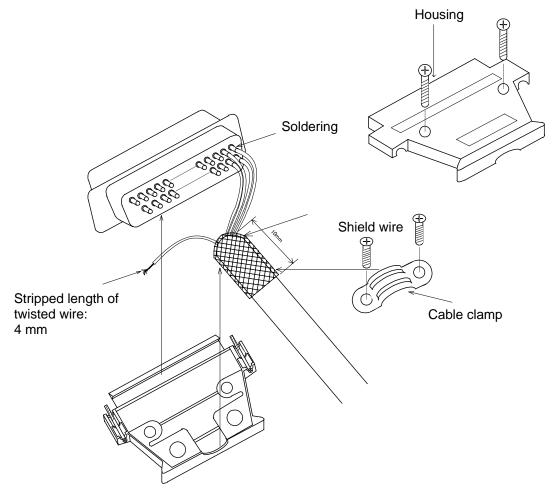
Note: The shield wire of the cable using a D-SUB connector is connected to the ground of the TS3100 robot controller through the housing. Completely connect the shield wire to the housing using the cable clamp.
