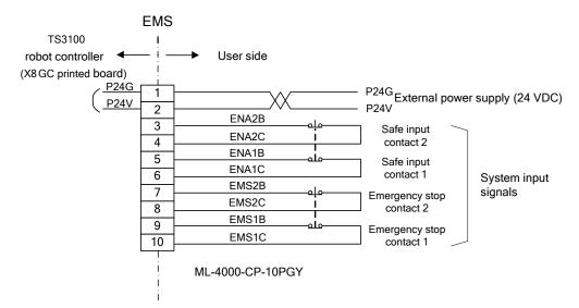
\* The system input signals "Emergency stop contacts 1 and 2 (linked 2-contact configuration)" and "Safe input contacts 1 and 2 (linked 2-contact configuration)" are non-voltage contact input.
