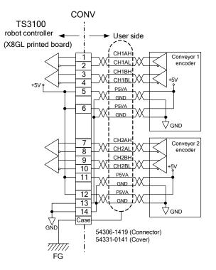
Fig. 10.2 Connection Between Incremental Encoders (when using internal power supply)
