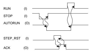
(3) Example of restarting the robot after servo OFF (emergency stop) Restart after servo OFF (emergency stop)
