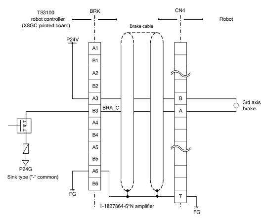
Fig. 13.1 Connecting motor brake signal cable
