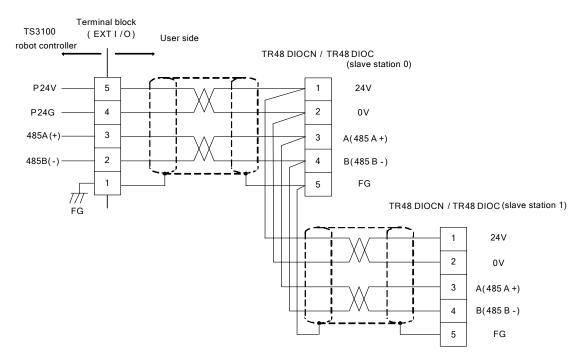
Fig. 7.2 Connection when relaying EXT-I/O cable
