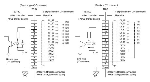
Fig. 9.1 Connection of trigger input signal cable
