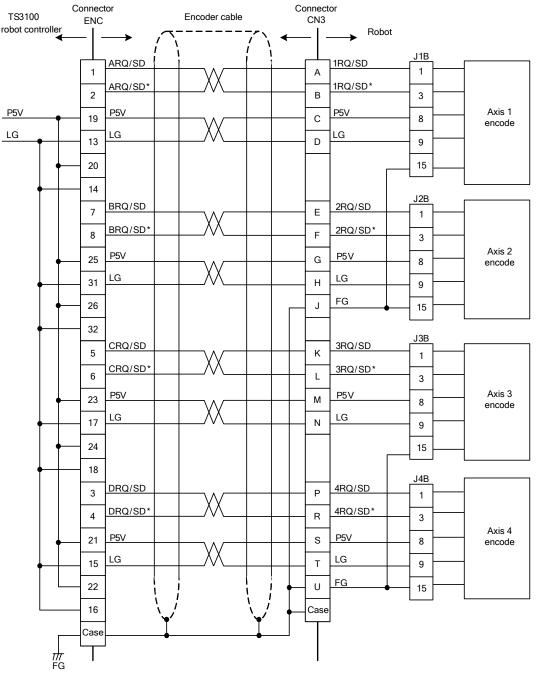
Fig. 3.3 Connection of encoder cables (SCARA type robot)
