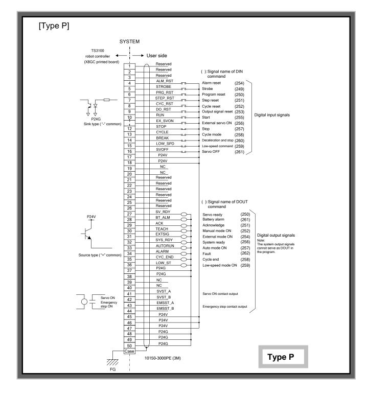
Fig. 4.6 Connection of external output signal cables (Type P)
