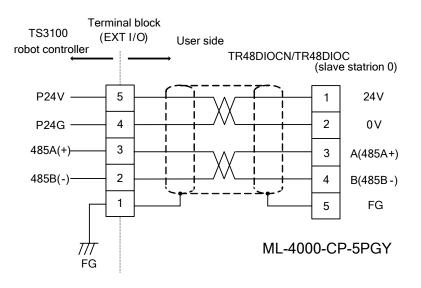
Fig. 7.1 Connection of RS-485 cable
