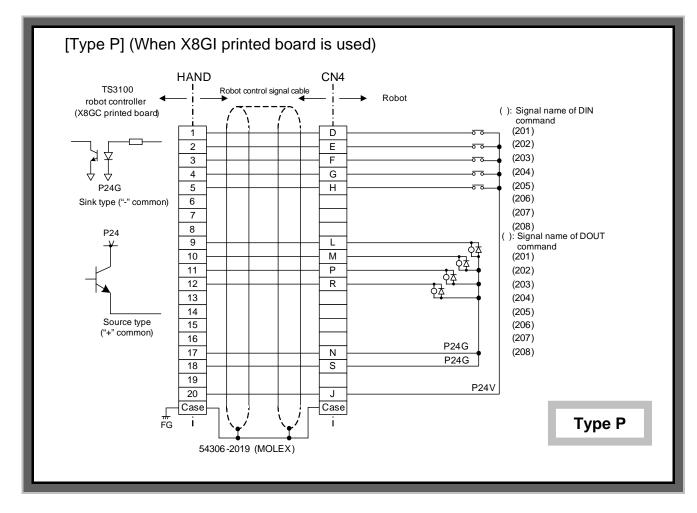
Fig. 3.6 Connection of robot control signal cable (Type P)
