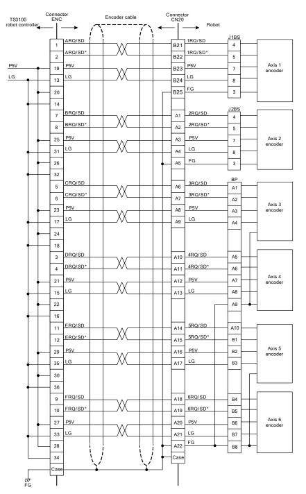
Fig. 3.4 Connection of encoder cable (6-axis robot)
