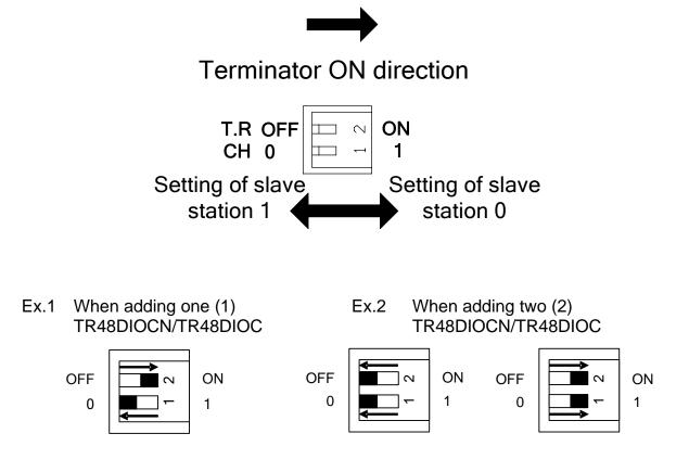
The slave station setting is already described above. Specify the slave station of TR48DIOCN/TR48DIOC to be used, according to the station number set in USER. PAR.
