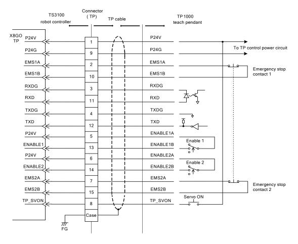
Fig. 6.1 Connection of TP1000 teach pendant I/O signals
