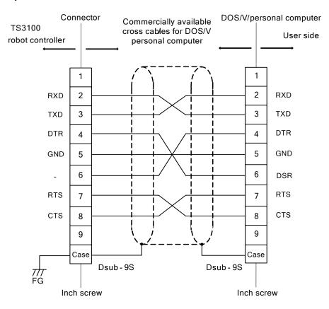
Fig. 5.1 Connection of serial I/O signals COM1, HOST, and TCPRG
