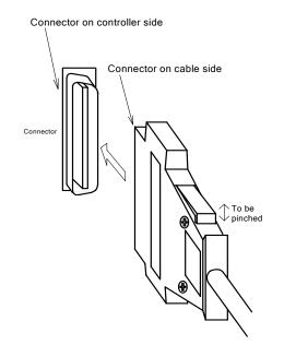
Fig. 4.8 Attaching and detaching external I/O signal cable (INPUT/OUTPUT)
