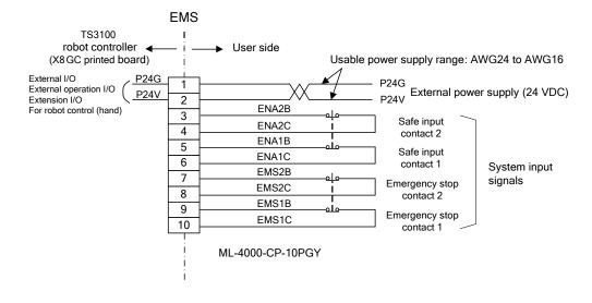
Fig. 14 Connecting external power supply
