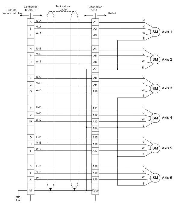
To connect the motors, use the attached cables.
