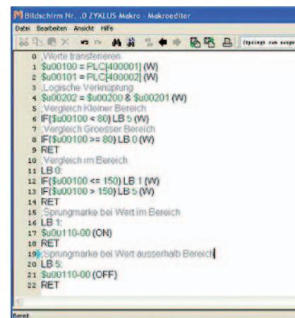
Easy to do in connection with a HAKKO touch panel: programming of basic PLC functions using the macro commands of the HAKKO V-SFT programming software.
