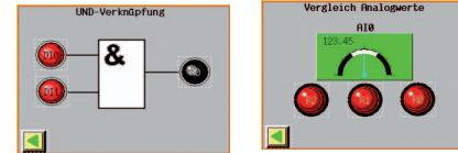
Visualization of the functional blocks as well as input and output data on the touch panel. Logging data may be stored on a CF memory card which can be installed in the HAKKO touch panel.
