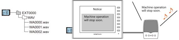
Playback of a WAV file saved to a storage device.
