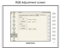
5. Press the [Save] switch to save the settings. Settings are stored in the flash ROM, so they will be retained even when the power is turned off and on again.
