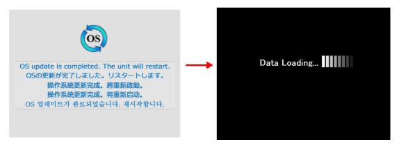
9. The "Loading from Storage" message is displayed again, and then the screen program saved to the storage device is written. When transfer is complete, the V9 series unit automatically switches to RUN mode.
