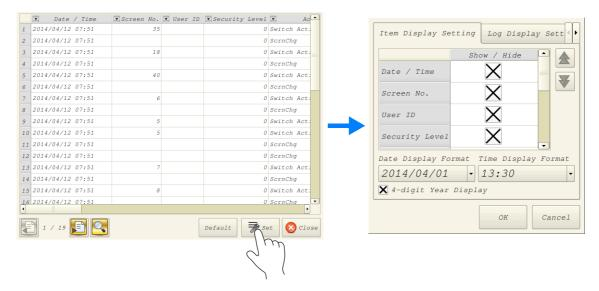
Select the [Log Display Setting] tab to check a list of items that can be displayed in the operation log viewer. Deselect the checkbox of items to hide and click [OK] to only display items with a selected checkbox.
